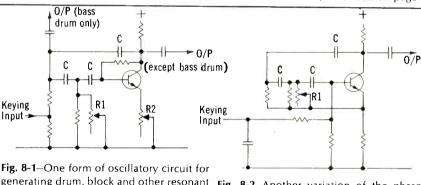
generating drum, block and other resonant percussive sounds. This circuit is adjusted not to oscillate, but to be active.
