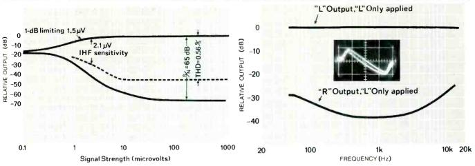
Fig. 3–Stereo FM characteristics of the Fisher Stereo FM/AM 500-TX receiver.
