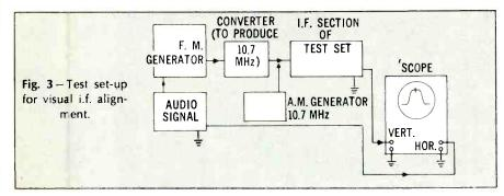
side" the frequency range, as such a setting will also result in a zero or near zero indication. The desired "zero" is the one which occurs between a positive and a negative swing of the meter. That is why it is easiest to perform this adjustment with a zero-center meter. Even a slight movement of the tuning adjustment slug to either side will cause a rapid movement of the meter pointer either to one side or the other, about zero center.
