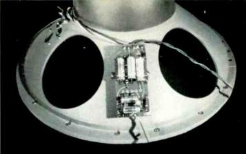
Fig. 1. The integrated-circuit amplifier mounted on a flattened leg of the Tannoy Dual Concentric loudspeaker, using the mounting clamp provided with the amplifier.
