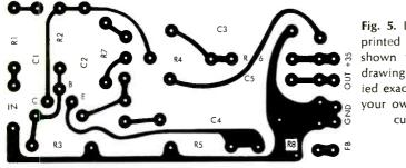
Fig. 5. Layout for the printed circuit board shown full size. This drawing may be copied exact size to make your own printed circuit board.
