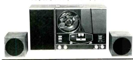
them is the reverse button to put the 20-Hz signal on the tape. To its left is a slide switch which changes equalization. One position is labeled  $7\frac{1}{2}$ , while the other is marked  $3\frac{3}{4}$ - $1\frac{7}{8}$ . The two slower positions use the same 120- $\mu$ sec equalization, so only two switch positions are necessary.
