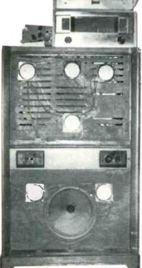
Fig. 3 – Author's loudspeaker system with grille cloth removed to show electrostatic speakers. At bottom is rear of the enclosure. The upper unit is a transistor amplifier; the lower unit is the power supply for electrostatic speakers.
