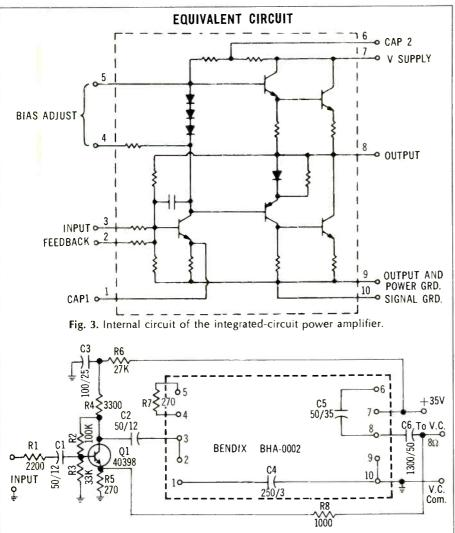
Fig. 4. Schematic of the completed unit with an additional stage to provide for more feedback to increase output into an 8-ohm load. The integrated-circuit amplifier is shown inside the dotted lines.
