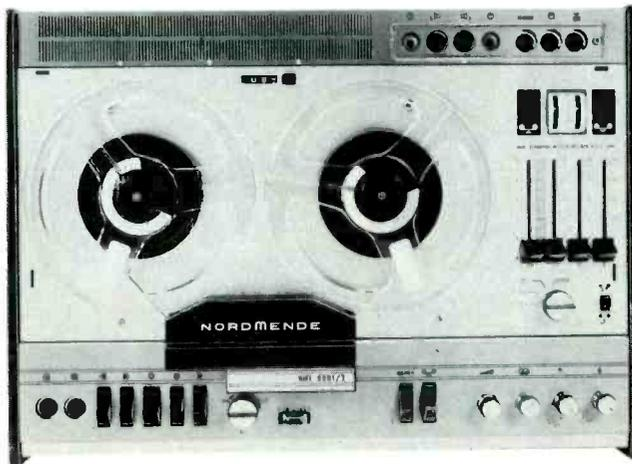
The NordMende Hi Fi 8001/T is a compact (but fairly heavy) 3-speed, 3-head, 3-motor, solid-state stereo tape recorder with two built-in speakers. The 4-track, 7-in.-reel-capacity unit, features sliding-type attenuator mixing facilities and a sleek (it's only 6-in. high), modern appearance. This is capped by a handsome, fitted, plexiglas cover that snaps into place over the brushed chrome and black panel, leaving only the connectors exposed.
