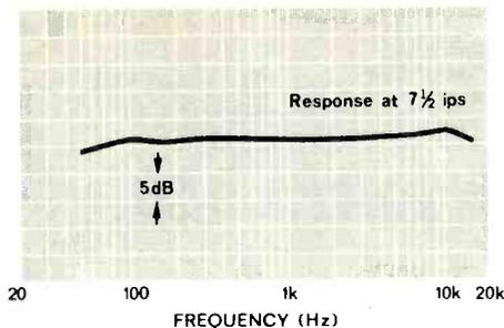
Fig. 2—Reproduce frequency response at two speeds of the NordMende 8001/T recorder.
