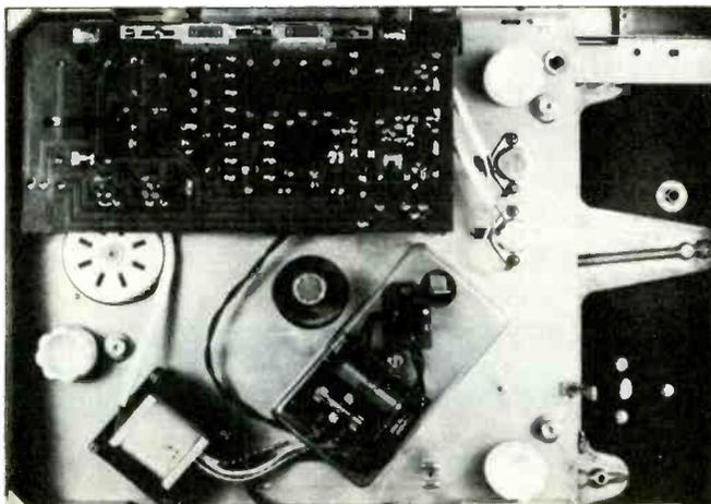
The motor drives the inner turntable through a small belt which isolates motor vibration from the turntable assembly. Below: the stroboscope seen through the window at the front of the panel. The photo was taken at  $33\frac{1}{3}$  rpm, and the line of light below the dots is the position of the 45-rpm dots. A sliding window adjusts for the line frequency in use.
