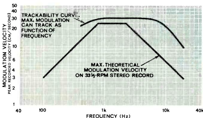
Fig. 3—Frequency response characteristic of phono cartridge with a specification of 20-20,000 Hz  $\pm$  2 dB.
