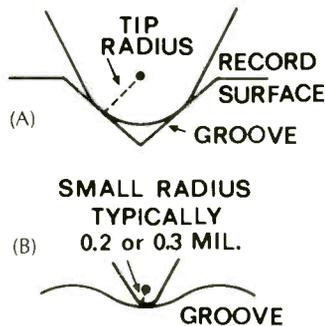
Fig. 7—(A) Illustrates a view of the stylus tip looking down the record groove. In (B), a view of an elliptical tip is shown looking at the record at an angle of 45 degrees (parallel to one groove wall).
