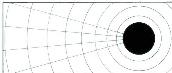
**Omnidirectional speakers** . . . most are omnidirectional only in the bass range . . . but notice that the vital high frequency tones, regardless of elaborate baffle systems, are perceptible only in a limited listening area.
