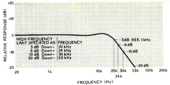
Fig. 5—Frequency-response curve showing several high-frequency limits, depending on how specified.
