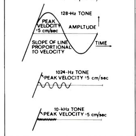
frequency signal. For many cartridges, we would find that there would be little difficulty encountered in reproducing the 1024-Hz tone. A somewhat better cartridge would be required to produce the low-frequency tone also. And an even better cartridge would be needed to reproduce all three signals faithfully.
