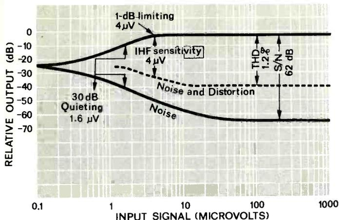
Fig. 3—FM characteristics of the Model 3200 Cortina tuner.
