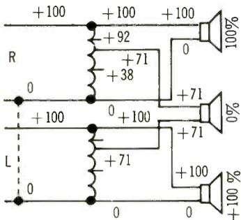
Fig. 1—Wrong! No voltage addition.
