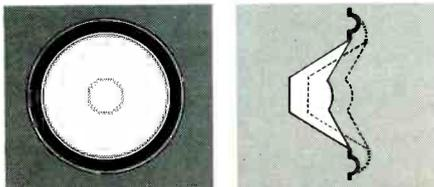
It suspends the woofer cone in University Sound's newest speaker system—the Project M. It allows the cone to make inch-long excursions and still maintain linearity accurate to within .001%. Try that on your woofer.
