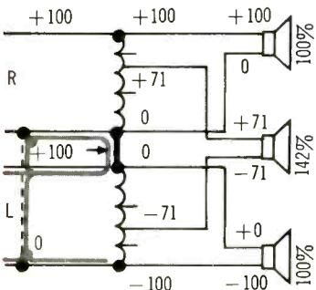
Fig. 2—Dangerous! Short circuit of one amplifier.
