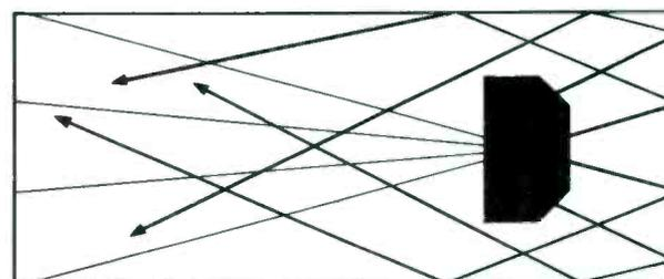
**Reflective speakers** . . . these can give a satisfactory illusion of presence and depth. However, these systems require an equalizer for flat response. This in turn generally requires the use of separate (and expensive) pre-amps and ultra-high-wattage power amps.
