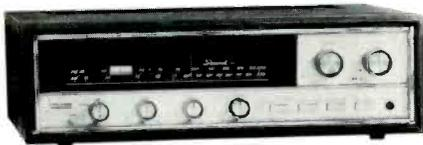
tion, main and/or remote speaker switching, and tape monitor. Other controls are loudness, bass, treble, balance, and variable FM muting for minimizing noise between stations. Phono input level can be adjusted with a three-position switch on the rear panel. Size is 16½" x 4½" x 12" deep. A walnut-grained, leatherette metal case or an oiled-walnut wood cabinet is available as an option.
