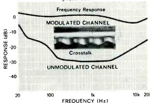
2. 15 to 20 dB separation at 10 kHz.
