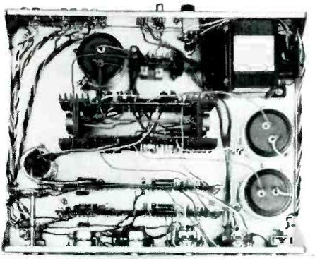
Open, uncluttered layout facilitates kit construction. Four etched circuit boards are factory assembled and tested.
