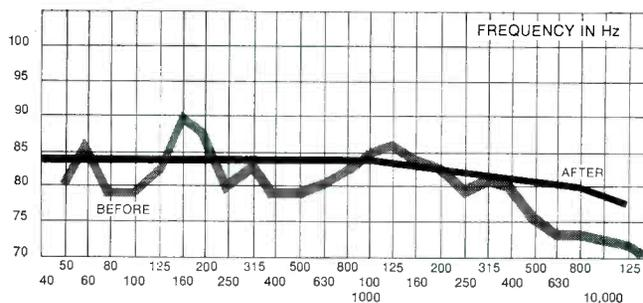
rejection filters. What's more, the *Acousta-Voicing* method is unique in its ability to insure integrity of transient response in the total system after equalization. The results of *Acousta-Voicing* are positive and dramatic. Witness the response curves as recorded by a precision sound level meter in
