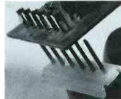
Snap-in printed circuit modular construction for reliability and ease of service.
