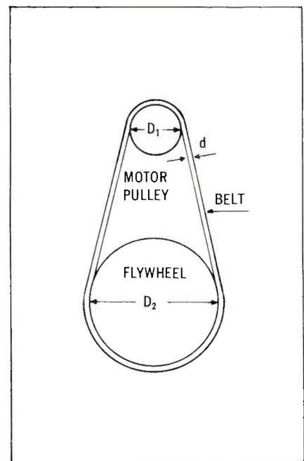
Fig. 2—Speed of a flywheel is not in inverse ratio to the diameters of motor pulley and flywheel, but has to take into account the thickness of the belt.
