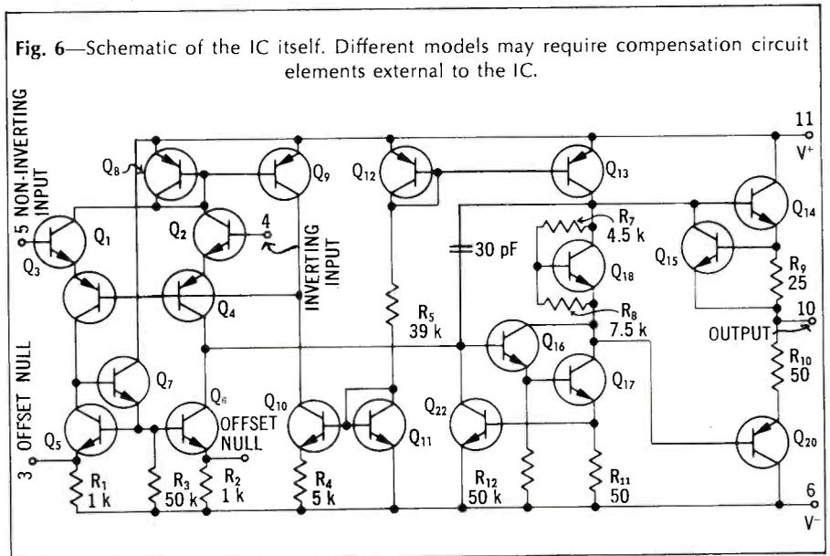
Fig. 6—Schematic of the IC itself. Different models may require compensation circuit elements external to the IC.
