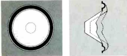
It suspends the woofer cone in University Sound's newest speaker system — the Project M. It allows the cone to make inch-long excursions and still maintain linearity accurate to within .001%. Try that on your woofer.
