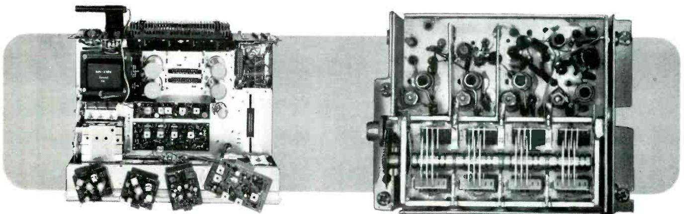
Sansui 4000's new printed circuit design features separate P. C. modules with plug-in multi-connectors for FM MPX, preamplifier and driver amplifiers, permitting faster more economical servicing.
