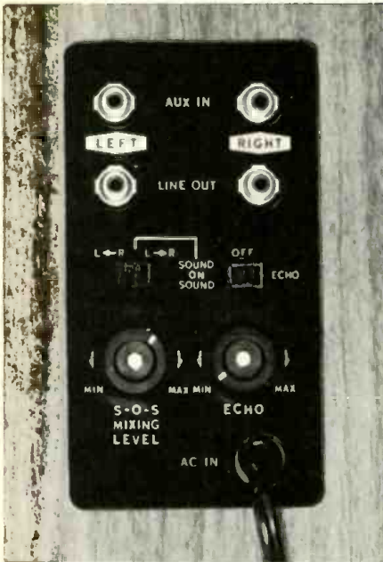
Fig. 2—Input and output connections are made in the recessed panel on the right side of the case, and additional switches and controls for sound-on-sound and echo are on the same panel.
