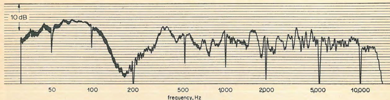
Fig. 5—Measured frequency response characteristic of a loudspeaker when touching the three surfaces in a corner.
