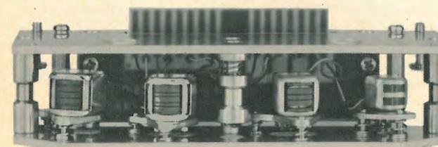
Fig. 2—Close-up view of head assembly.
