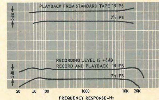
Fig. 4—Response curves for playback of standard tapes and for recording and playback.
