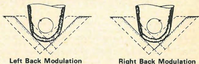
Fig. 1—The two circular modulations of the SQ system.
