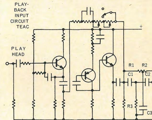
Fig. 3—Playback input circuit (one channel only).
