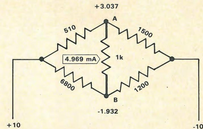
Fig. 2—Bridge with resistances calculated.
