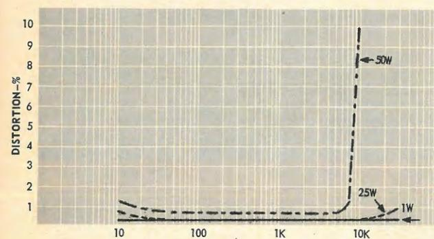
Fig. 7—Distortion vs. frequency at various power levels.
