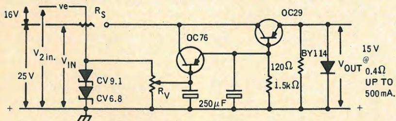
Fig. 5—A simple bench power supply circuit, with rudimentary control, effective over a limited range of values.
