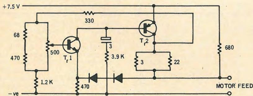
Fig. 6—A variant (by B. R. C. Ltd.) on the supply and motor regulation circuit of the Philips cassette portable shown in the Jan., 1971 issue of *AUDIO*, p. 28.
