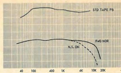
approached. Frequency response measured within  $\pm 2\frac{1}{2}$  dB from 40 to 13,000 Hz in the flat position, while the noise suppressor rolled off response about 10 dB at 10,000 Hz. The auto-eject feature was judged useful for those who will use the unit for playing recorded tapes consistently, and it is undoubtedly a convenience in normal use. We had relatively little information about this machine, so everything described or charted is the result of inspection and measurement.
