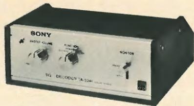
This decoder is designed to be used with the recently announced Columbia SQ quadrasonic system, which permits four channels to be reproduced from a two-track source. Also announced is the SQ-444 from Columbia Masterwork, which includes decoder-receiver, automatic turntable, and four speakers.
