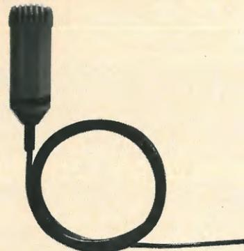
This dynamic microphone uses double-wall construction with two separate cases, one nested inside the other and insulated with highly compliant rubber. The unit weighs 8 oz., is 2½ in. long, and has a diameter of less than one in. This omnidirectional microphone has a specified frequency response of 90 to 10 kHz and is matched for low impedance inputs. Price, \$133.
