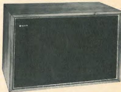
The Criterion 4X speaker system features a four-speaker design, with a 12-in. bass speaker, a 5-in. mid-range, a 3-in. for the 5000-to-10,000 Hz range, and a 1½-in. super tweeter for frequencies up to 20,000 Hz. Impedance: 8 ohms. Size: 22 × 14½ × 11½ in. Price: \$69.95.
