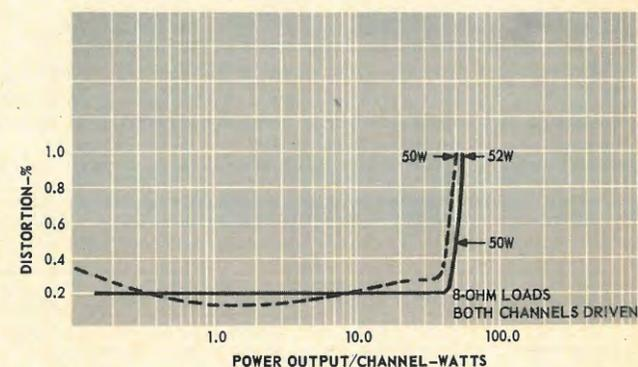
Fig. 5—Distortion characteristics.
