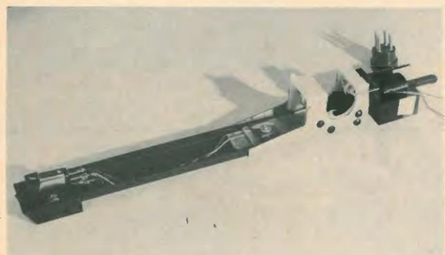
**Fig. 1**—Underside of arm, showing nylon guide rollers, counterweight, and the four-contact plug carrying the pickup output. Plug inserts in matching receptacle on chassis, and four fine wires carry the signal from the cartridge with a minimum of drag on the arm.
