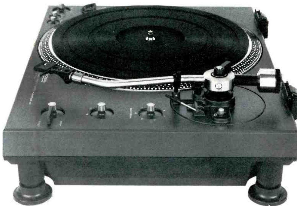
level, while the DIN B (and the DIN A for that matter) use a 10 cm/sec level so these figures will come out some 9 dB higher at the outset. As the rumble components are mostly in the 25 to 40 Hz band, the DIN B figure would be around 75 dB—in other words 5 dB better than the specifications. (If you think this sounds like a plea for standardization, you would be right!)
