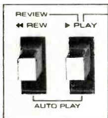
**Auto Play and Auto Stop Function.** This lets the tape play all by itself. With the PLAY and REWIND keys pressed at the same time, the tape will rewind to the beginning of the cassette, stop, and automatically begin playback. The Auto Stop mechanism automatically switches the tape off at the end—so it protects the tape deck and your tapes.
