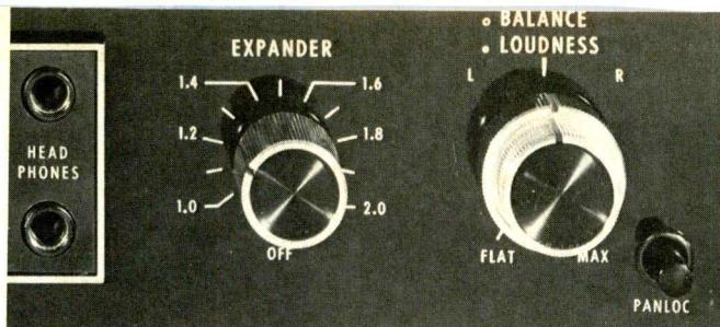
Fig. 1—Close-up view of the expander control.
