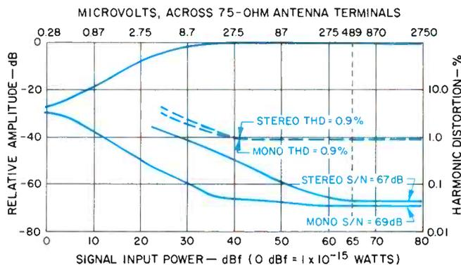
**Fig. 2—Distortion vs. frequency for the FM section of the CA-9500 tuner.**
