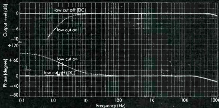
Gain, Phase vs. Frequency Response, SE-9060 Amp.
