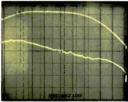
**Fig.3— The FM response (including de-emphasis) and stereo separation.**
