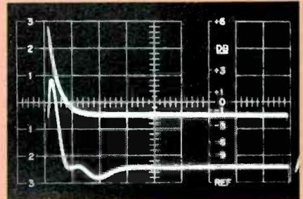
Fig. 5—Preamp output (top) with 1-kHz square-wave input and a +10-dB boost at 10 kHz with the tone control. Equalizer output (bottom) with the 1-kHz square-wave input and filters set to match the preamp frequency response.
