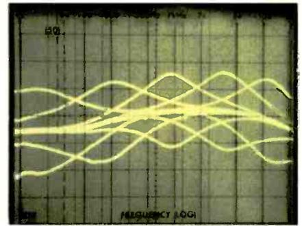
**Fig. 4— The range of control for the equalizer levers on the Motorola EQB-3000 equalizer/booster. (One vertical division equals 10 db.)**
