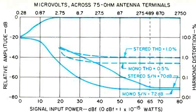
Fig. 1—Mono and stereo quieting and distortion characteristics for the FM section of the Sanyo FT-1490A.
