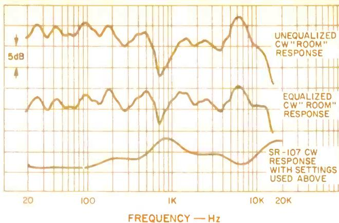
Fig. 3—Equalization of room-like response.
