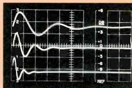
Fig. 2—Equalizer output with 170-Hz square-wave input with a 12-dB boost successively in 1800- (top), 3600- (middle), and 7200-Hz filters.
