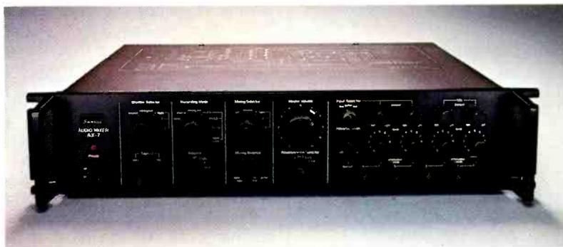
20dB input level attenuators on the 4 main inputs. Reverb is included, as well as circuits for 4-channel, equalization and noise reduction. Record the sounds you create on up to 3 tape decks.
