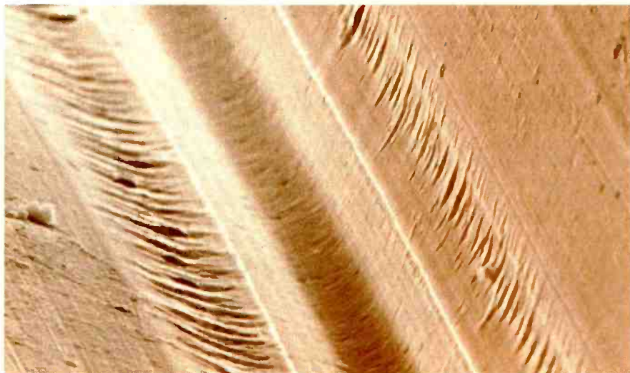
Fig. 13 — Magnified view of single groove of untreated record after 100 playings.
