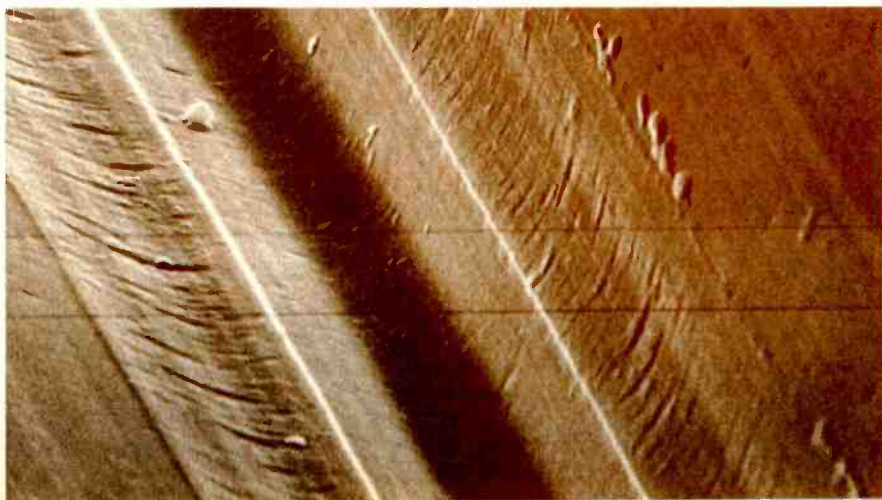
Fig. 14 — Magnified view of single groove of Permostat-treated record after 100 playings.
