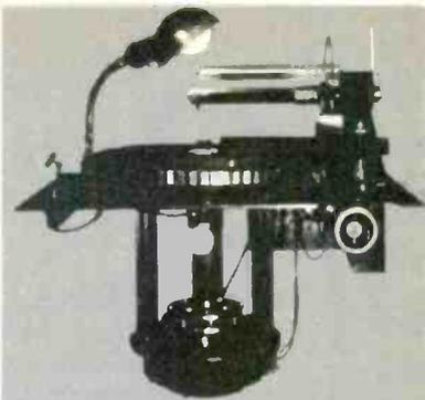
In 1939, while many turntable manufacturers were trying to make the transition from horn phonographs to electrical record players, Denon developed its first direct-drive turntable (shown above). Denon engineers discovered that only a direct connection between motor and platter—free of the pulleys or belts found in more primitive drive mechanisms—could completely eliminate speed fluctuations that obscure musical detail.
