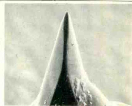
**Fig. 1—Lateral SEM view of the van den Hul stylus in the MIT-1. The dark area in the center of the stylus, from the tip to where it begins to widen, is the actual groove contact area, which is 143  $\mu$  long by 10  $\mu$  wide. (x300 magnification.)**
