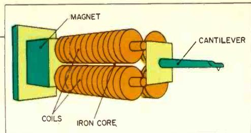
Fig. 4 — Simplified drawing of a variable-reluctance cartridge. (After Osawa's "A Consumer Guide to Phono Cartridges.")
