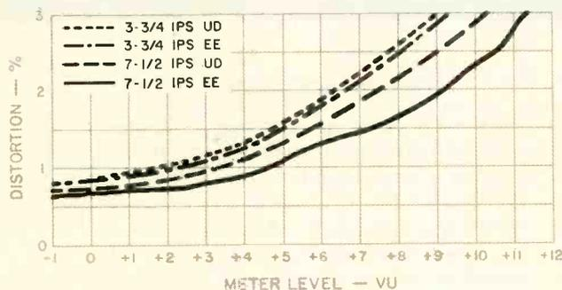
**Fig. 3 — Distortion and headroom at 1 kHz.**
