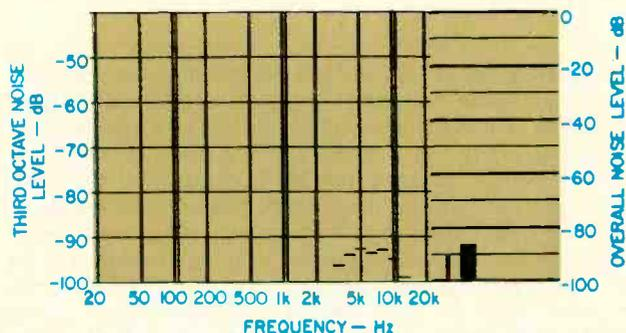
**Fig. 6 — Have you ever seen this sort of S/N figure for a "tape recorder" before? The 86.1 dB (below 0-dB record level) is actually the residual noise of the test unit!**
