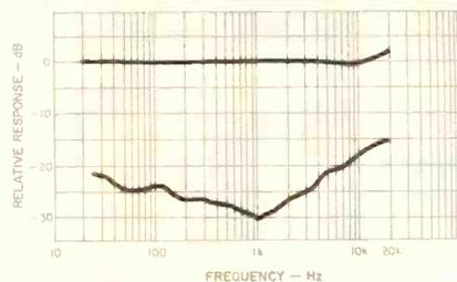
Fig. 1 — Frequency response and separation.
