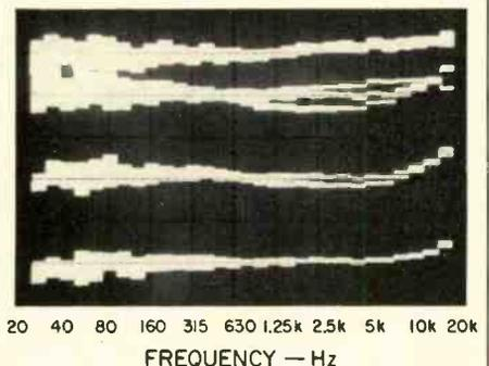
Fig. 1—Top, Type I tape responses. Second, Type II tape responses. Third, Type III tape responses. Bottom, Type IV tape responses. See text for discussion. (Vertical scale: 5 dB/div.)
