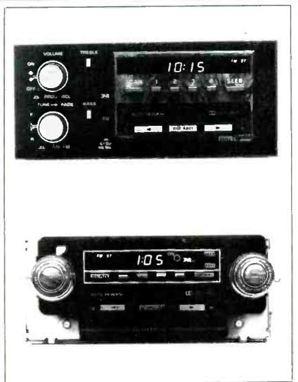
*Fig. 4—The matching Delco receivers have both DNR and Dolby. Note the absence of a balance control.*
