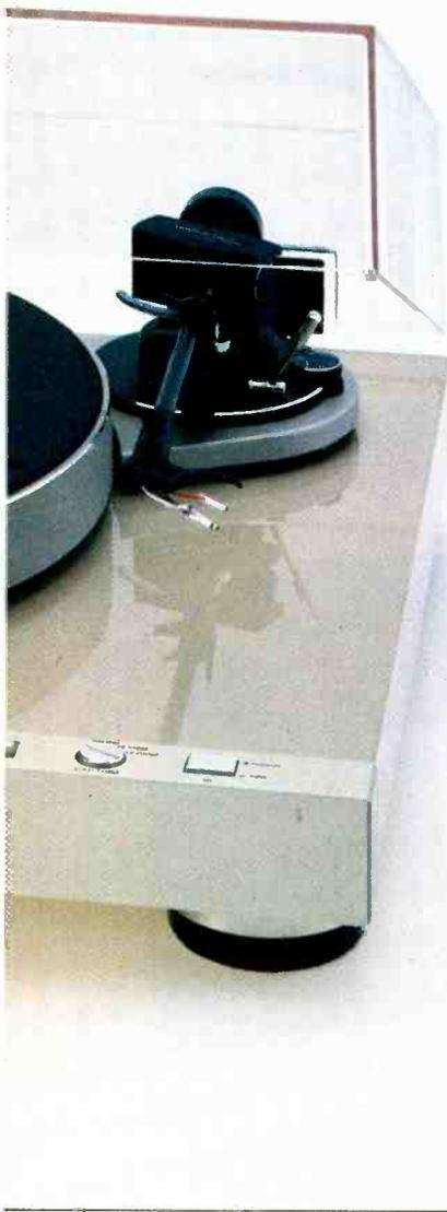
cause resonances. The arm is a low-mass type (only 8 grams) constructed from tubular aluminum and measuring 8.9 inches from pivot to stylus. Micro-race bearings are employed, and the headshell, which is made from light-
