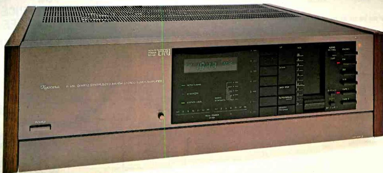
Kyocera and Cybernet are corporate relatives, and this time the corporate decision has been to bring out a line of receivers (or tuner-amplifiers, if you insist) under the Kyocera brand name. The top unit in that line is the Model R-851, a frequency-synthesized, full-featured AM-FM tuner combined with an equally full-featured preamplifier-power amplifier capable of delivering in excess of 85 watts per channel into 8-ohm loads.
