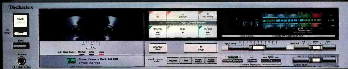
dbx is effective because it compresses a musical signal so its dynamic range is cut in half. When the tape is played back, the original dynamic range is restored, but the noise level is pushed below the level of audibility.
