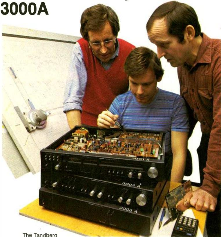
The Tandberg TPT 3001A Programmable FM Tuner, like all the other members of the Series 3000A, features discrete components — not integrated circuits — individually selected to meet ideal performance parameters.
