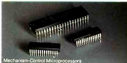
The microprocessors determine drive motor speed and direction to provide flawless auto-reverse operation. With this "intelligence" in control of DRAGON's mechanism and circuitry, several unusual features are possible: Auto Record Pause, Easy Cueing, Punch-In Recording, and Memory Stop/Play.
