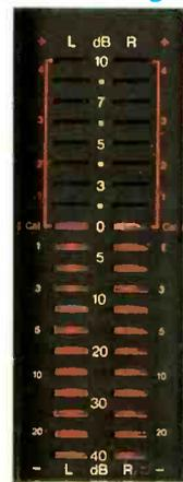
DRAGON's peak-reading electronic meters span a full 50-dB range — from -40 dB to +10 dB — with 20 LED segments per channel. They are fast responding but hold the peak reading momentarily so they are easier to read. Being completely electronic, they are free of "pointer lag" and "overshoot." These precision instruments automatically increase sensitivity by 20 dB in the calibration mode to improve the precision of the adjustments.
