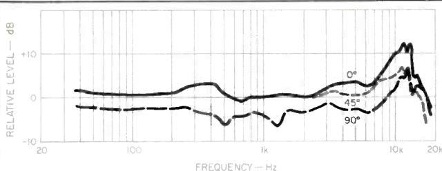
**Fig. 3—Frequency response vs. angle of PZM-180 on pseudo-infinite baffle.**
