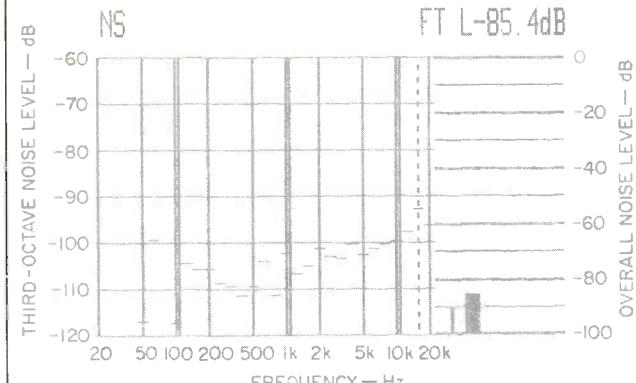
**Fig. 6—Unweighted S/N analysis, without added dither.**
