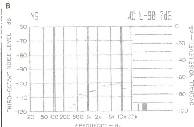
**Fig. 5—S/N analysis with Digital Time Lens adding dither, both unweighted (A) and A-weighted (B).**
