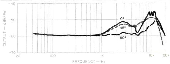
**Fig. 4—Frequency response vs. angle of PZM-180 without baffle.**
