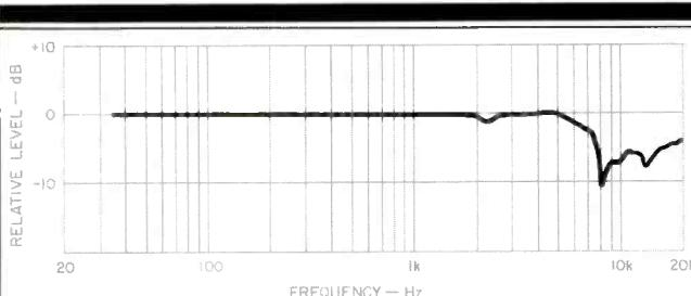
**Fig. 5—Effect of windscreen (logo side down) on frequency response, with microphone mounted on pseudo-infinite baffle.**
