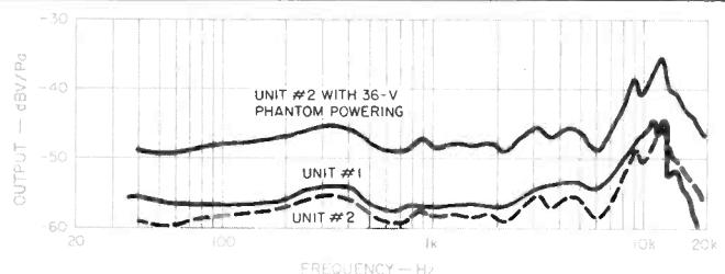
**Fig. 2—Frequency response of both PZM-180 microphones, on pseudo-infinite baffles. Top curve: 36-V phantom power; lower two curves, 1.5-V battery power.**
