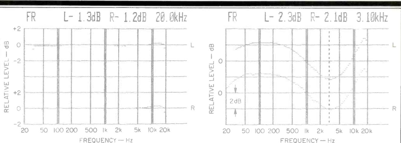
**Fig. 1—Frequency response, left (top) and right channels, with Digital Time Lens off.**
