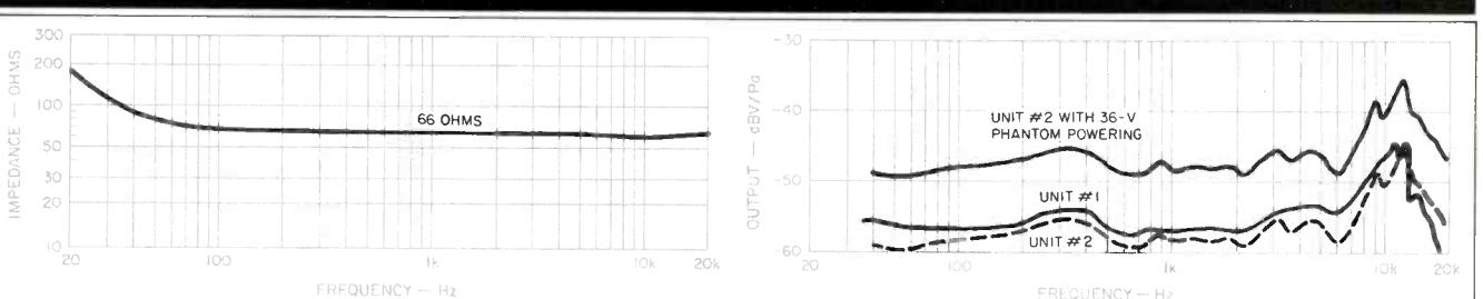
**Fig. 1—Impedance vs. frequency was identical for both PZM-180 samples (1.5-V power).**
