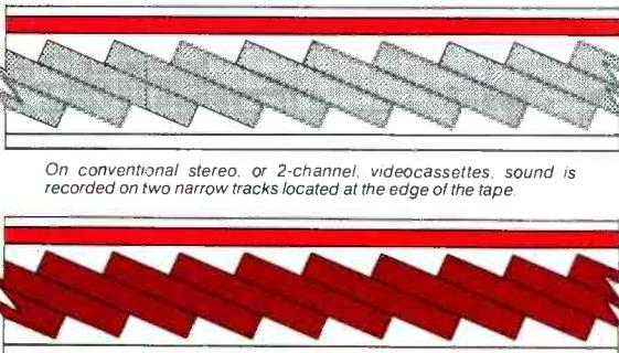
On conventional stereo, or 2-channel, videocassettes, sound is recorded on two narrow tracks located at the edge of the tape.
