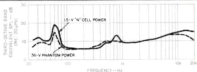
**Fig. 6—Noise level vs. frequency (microphone unit No. 1). Overall noise level measured 24 dBA or 28 dB unweighted.**
