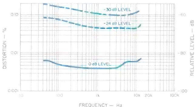
**Fig. 4—THD vs. frequency at three signal levels.**
