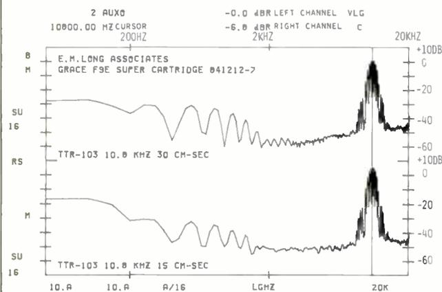
**Fig. 11—** Spectrum of distortion products for 30- and 15-cm/S signals shown in Fig. 10. Level at
