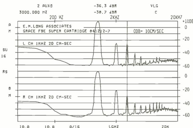
**Fig. 9—Spectral components of 1-kHz signal shown in Fig. 8. Level of third harmonic (3 kHz) is 1.6% in the left channel and 1.1% in the right (1.0% equals -40 dB).**
