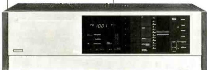
Dolby Surround, for videos and movies) plus stereo (bypass) and mono settings. Built-in, rear-channel amplifiers deliver 40 watts per channel, and a switchable, center-front channel output is also included. Price: \$549.95; optional wireless remote control, \$75.
