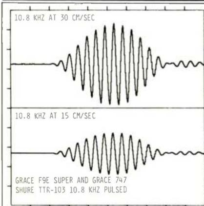
**Fig. 10—** Arm/cartridge output at 30 and 15 cm/S, 10.8-kHz pulse test. Note the small amount of asymmetry and absence of compression even at 30 cm/S, a very high level.
