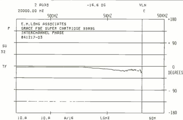
**Fig. 7—Interchannel phase of tonearm and cartridge as a function of frequency (B & K 2011, band 7, pink noise). Phase difference at 20 kHz is 16.6° (2.3 μS).**
