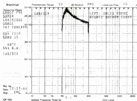
**Fig. 2—Low-frequency tonearm/cartridge resonance is at 6 Hz, with a Q of 4.6, using B & K 2010 test record.**
