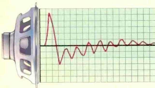
The illustration shows a conventional cone "ringing" long after the electrical impulse from the amplifier has ended. It's known as Time/Energy distortion.
