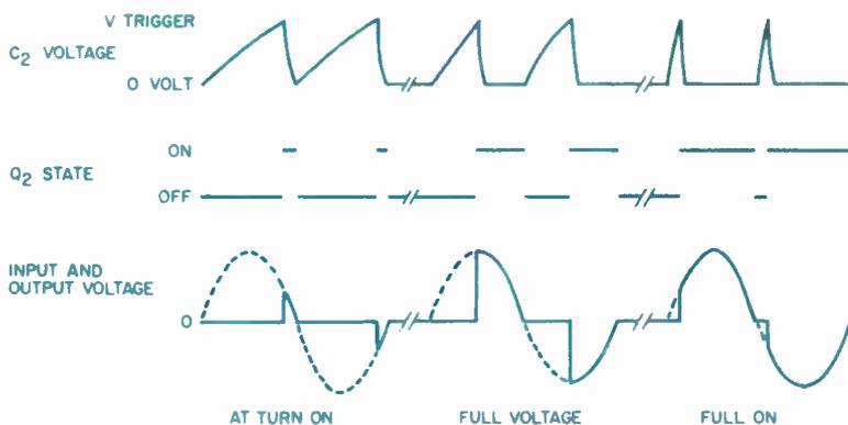
Fig. 2—Timing diagram. Transistor Q1 (not indicated) turns on when C2's voltage (upper trace) is higher than Q1's trigger voltage; this discharges C2. Transistor Q1 also triggers triac Q2 (middle traces), which delivers
