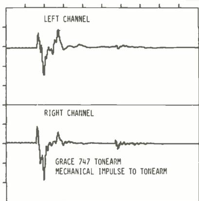
**Fig. 4—** Output of tonearm due to mechanical impulse applied to arm tube, with arm on rest but not locked. Total time period is 20.47 mS.
