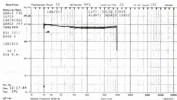
**Fig. 3—Tonearm resonance check, using slow sweep from 20 Hz to 1 kHz.**
