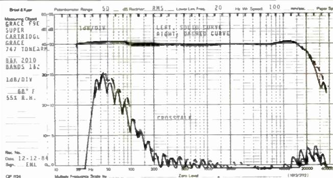
**Fig. 1—Frequency response and interchannel crosstalk of arm and cartridge, using B & K 2010 test record.**
