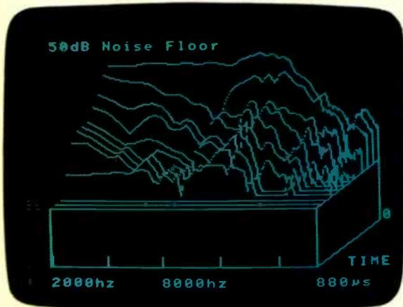
Computers provide information that conventional tests cannot. The display above shows how the various frequencies the driver produces fade away after the signal is cut off.
