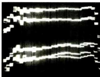
**Fig. 1—Record/playback responses for two tapes, at two levels; response with Dolby C NR is superimposed on response without NR in each case (the upper trace of each overlapped pair is with NR). From top to bottom: Maxell UD-XL I (Type I) at Dolby level, TDK SA (Type II) at Dolby level, Maxell UD-XL I at  $-20$  dB, and TDK SA at  $-20$  dB. Note the close match between responses with and without Dolby C NR at Dolby level, and the less close match at  $-20$  dB. See text. (Scale: 5 dB/div.)**
