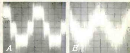
A. Ultra-low-level (4 significant bits) 1kHz signal, as reproduced by conventional CD players.
