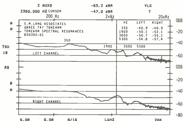
**Fig. 5—** Spectral analysis of tonearm output due to mechanical impulses, with 16 impulses applied
