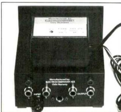
step-up devices available, the moving-coil cartridge was usually touted as being superior to the moving-magnet and moving-iron types. Finally, a cult developed that even today insists the moving-coil cartridge provides superior reproduction of recorded music. Meanwhile, further research has brought forth superior transformers and pre-preamplifiers, but at prices (\$1,000 and up) that few audiophiles can afford.
