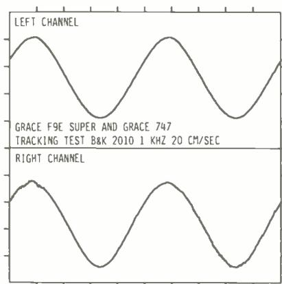
**Fig. 8—Tracking of arm and cartridge at 1 kHz, 20 cm/s. Note slight mistracking at this level.**
