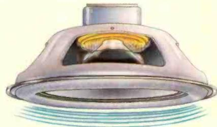
A conventional driver's cone rings like a bell. The voice coil motion makes the cone flex and store energy which is later released causing Time/Energy distortion.
