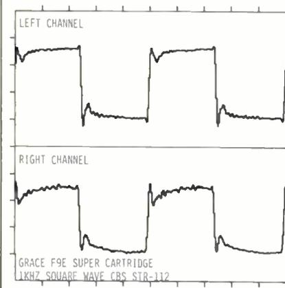
**Fig. 12—** Arm/cartridge output for 1-kHz square wave, CBS STR-112 test record.
