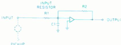
Fig. 1—Partial circuit diagram of the MC-2 pre-preamp.
