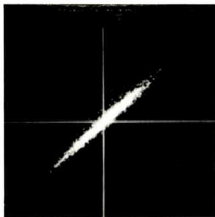
**Fig. 6—** Interchannel phase of cartridge, using B & K 2011 test record, band 7, pink noise.
