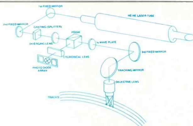
A typical LaserVision videodisc optical system, such as this, is similar in principle to a CD player's.
