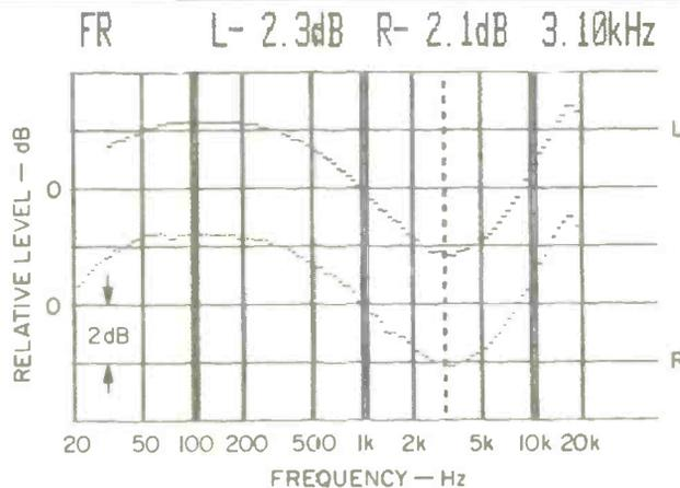
**Fig. 2—Same as Fig. 1 but with Time Lens on. Bass treble dips are  $-2.1$  to  $-2.3$  dB at 3.1 kHz. Note also treble peak just below 20 kHz.**
