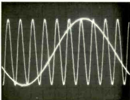
Fig. 9—Two-tone phase-test signal (200 Hz and 2 kHz).
