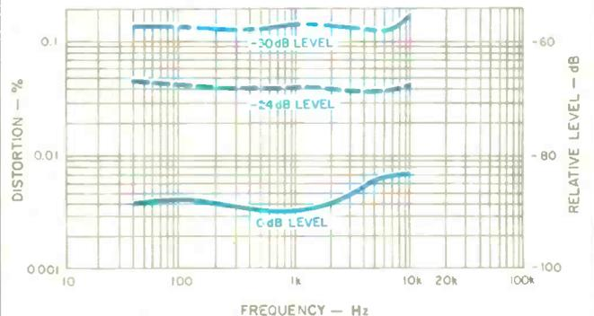
Fig. 2—THD vs. frequency at three output levels.
