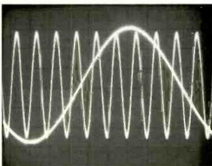
Fig. 8—Phase-error check using 2- and 20-kHz tones; see text.
