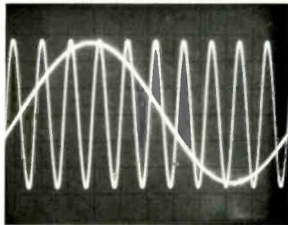
**Fig. 9—**Two-tone phase-test signal (200 Hz and 2 kHz) with Digital Time Lens off.
