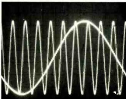
Fig. 8—With a 200-Hz signal on left channel and a 2-kHz signal on right (A), little or no phase shift is observed. Using 2- and 20-kHz signals, considerable time delay is noted (B).
