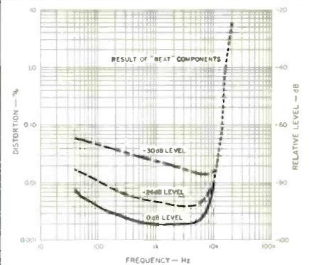
Fig. 3—Harmonic distortion vs. frequency, at three signal levels.
