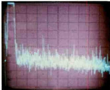
**Fig. B9—With dither added, overall noise level increases, but distortion components vanish below the noise floor.**
