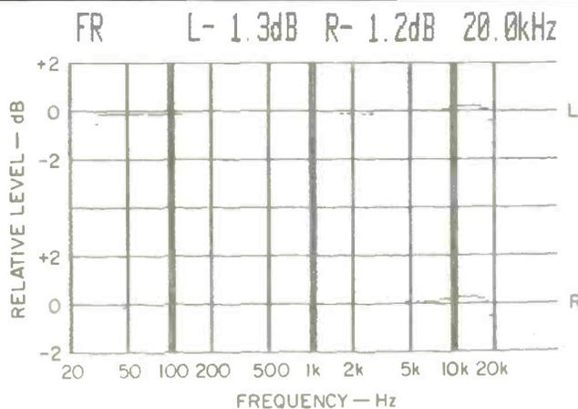
**Fig. 1—Frequency response, left (top) and right channels, with Digital Time Lens off.**
