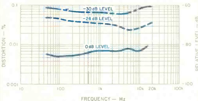
Fig. 3—THD vs. frequency at three output levels.
