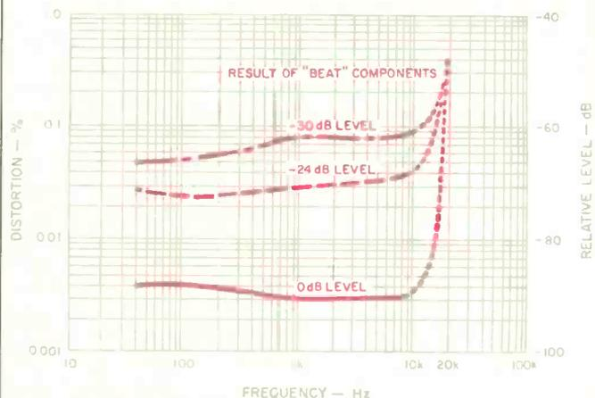
Fig. 3—THD vs. frequency at three signal levels.
