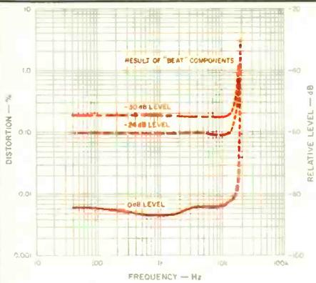
**Fig. 2—THD vs. frequency, at three output levels. Dashed portions of curves (beyond about 16 kHz) are “beat” components rather than distortion (see text).**
