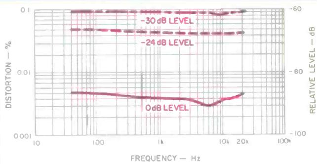
**Fig. 2—THD vs. frequency at three signal levels.**
