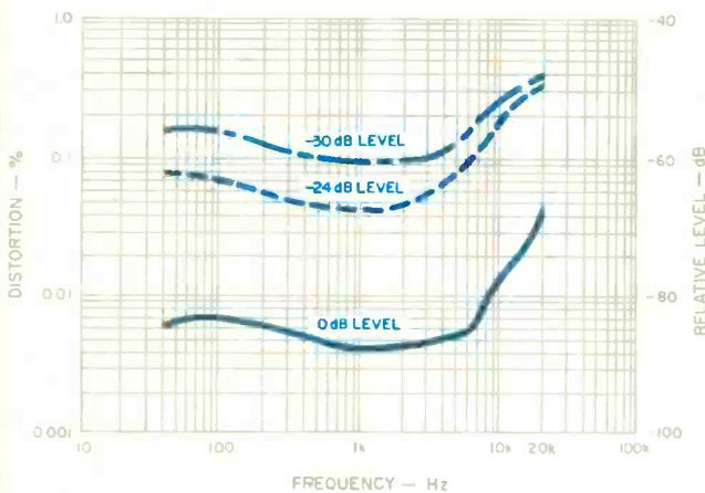
Fig. 2—Distortion vs. frequency at three recorded levels.
