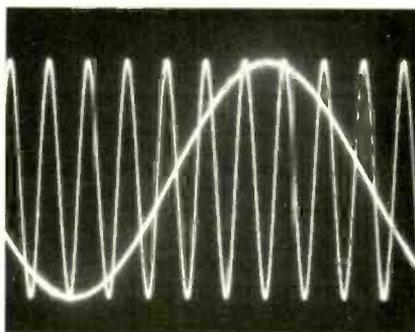
Fig. 8—Two-tone phase test using 2- and 20-kHz signals indicates that they are not reproduced with the proper time relationship.
