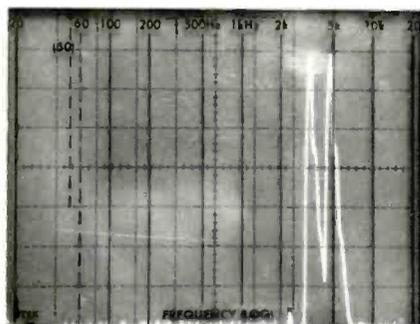
Fig. 5—IHF twin-tone IM test (14 and 15 kHz) showed 0.03% distortion—more than usual, but still minute.
