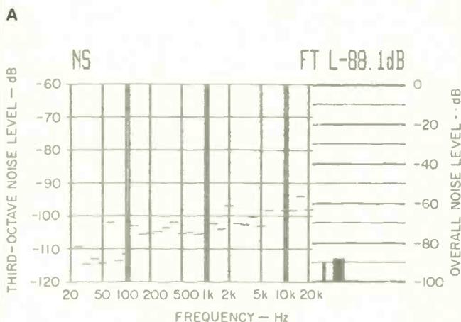
**Fig. 2—Unweighted S/N analysis in 14-bit mode (A) and 16-bit mode (B).**
