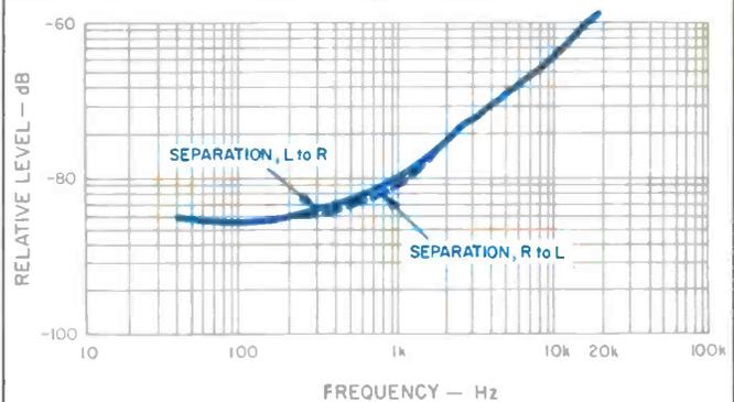
Fig. 10—Separation vs. frequency.
