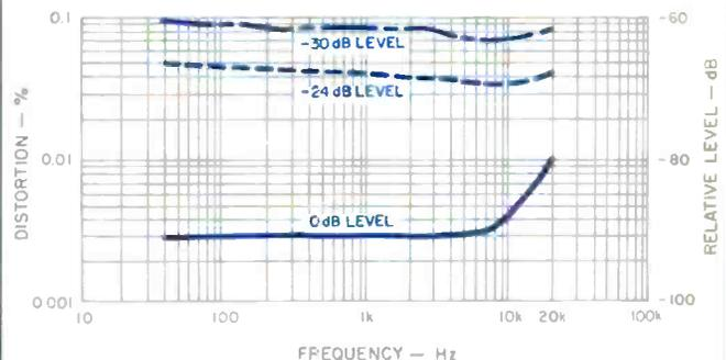
Fig. 2—THD vs. frequency at three signal levels.
