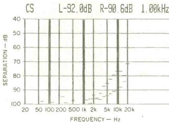
Fig. 5—Separation vs. frequency.
