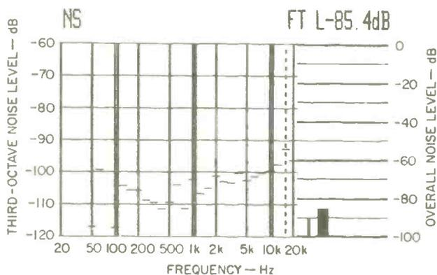
**Fig. 6—Unweighted S/N analysis, without added dither.**
