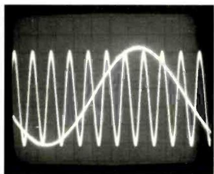
Fig. 8—Phase-error check, using tones of 2 and 20 kHz.
