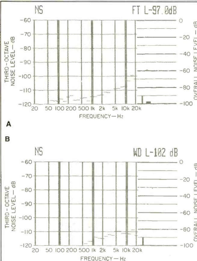
Fig. 5—S/N analysis, unweighted (A) and A-weighted (B).
