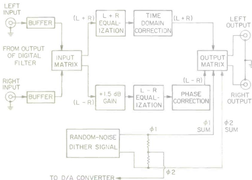
**Fig. B5—**Block diagram of the Carver Digital Time Lens.
