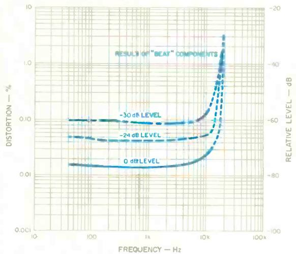
Fig. 2—THD vs. frequency at three signal levels; see text.
