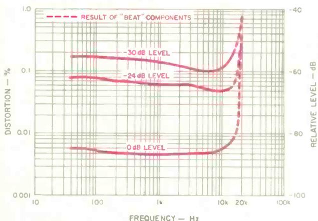
Fig. 3—THD vs. frequency at three signal levels. (High-frequency dashed lines indicate super-audible beats; see text.)
