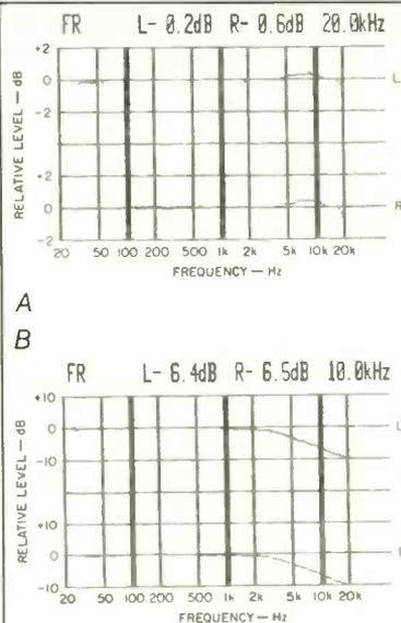
Fig. 1—Frequency response, left (top) and right channels, with high-cut filter off (A) and on (B). Note change of vertical scale, from 2 dB/div. (A) to 10 dB/div. (B).
