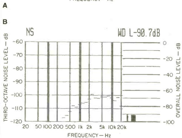
**Fig. 5—S/N analysis with Digital Time Lens adding dither, both unweighted (A) and A-weighted (B).**
