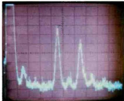
**Fig. B8—Spectrum analysis of waveform shown in Fig. B6 shows high level of harmonic distortion components.**
