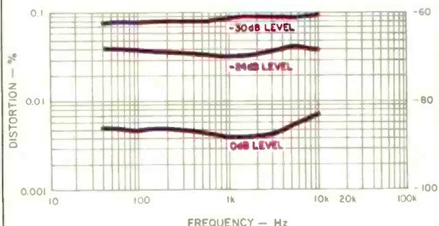
Fig. 4—THD vs. frequency, using low-pass filter, at three signal levels.
