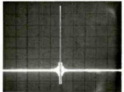
Fig. 7—Two-tone phase test (200 Hz left channel, 2 kHz right).
