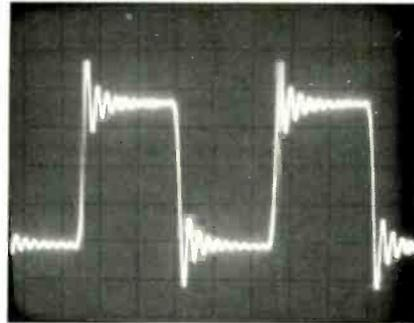
Fig. 5—Reproduction of a 1-kHz square wave.
