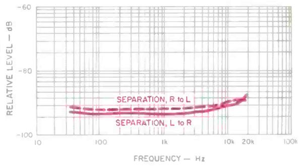
**Fig. 3—Separation vs. frequency.**
