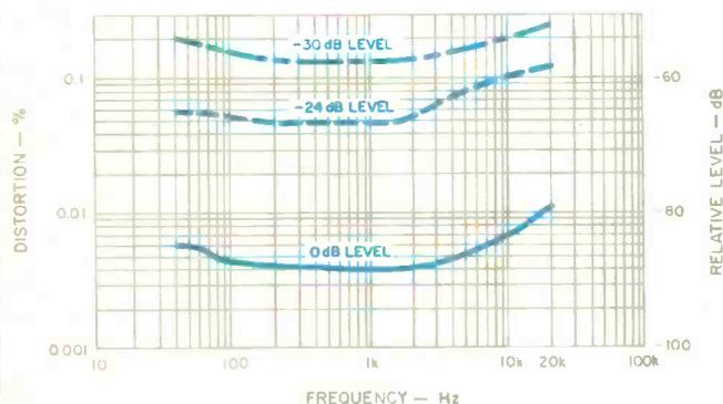
Fig. 2—THD vs. frequency at three signal levels.
