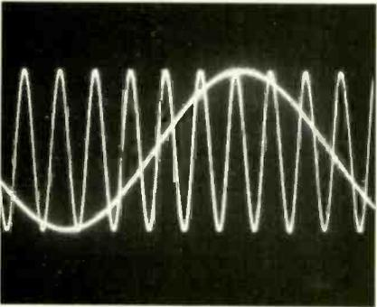
Fig. 8— Two-tone phase-test signal (200 Hz and 20 kHz).
