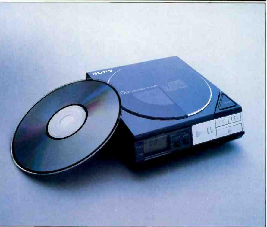
what track is being played, how much time has elapsed on a given track, and, at the press of a button, the amount of time remaining on the entire disc and the number of tracks remaining. In addition, there is a battery condition indicator and two other LCD indications: One for "AMS" (Automatic Music Sensor) and the other for music "Search" or audible fast-scanning of a disc's contents.
