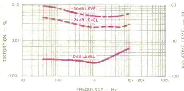
Fig. 2—Distortion vs. frequency, at three signal levels, using low-pass filter (see text).
