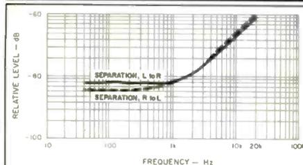
Fig. 5—Separation vs. frequency.
