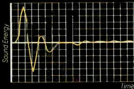
*A speaker with a T/E technology cone stops producing sound almost immediately after the signal ends.*
