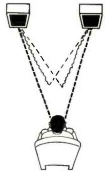
Special circuitry analyzes and generates a third set of impulses which are calculated to exactly cancel the second, muddying set. You don't hear this audio signal. It is, instead a sort of mirror image of the extra sonic arrivals, but out of phase so that one set "neutralizes" the other. Thus restoring perception of differences in depth and ambience in the stereo image which are "masked" in ordinary stereo playback.
