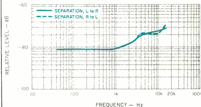
Fig. 5—Separation vs. frequency, from left to right and from right to left channels.
