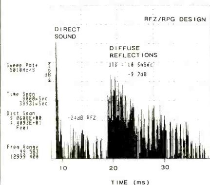
Fig. 8B—Energy-time curve of Pisha's listening room of Figs. 6 and 7 after RFZ/RPG treatment, showing much improved response. An initial time-delay gap of 10 mS was created with an RFZ 24 dB below the direct sound. The reflection pattern consists of a dense, uniform, exponentially decaying sound field.
