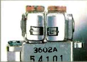
With typical "combination" heads, slight azimuth misalignment between the heads is vir-
