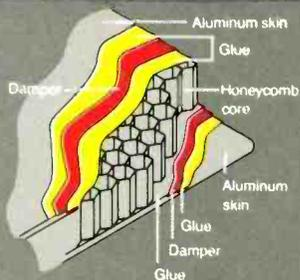
stiffer than ordinary diaphragms. This high rigidity makes it possible to design a flat driver that is free of "cavity effect." The APM driver diaphragm is also well damped and exhibits virtually no internal resonances that can alter reproduction accuracy.
