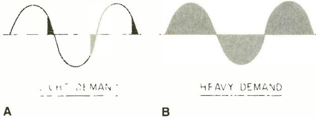
**Fig. 1—With light demand, Phase Control Regulation delivers power-supply voltage for only a portion of each a.c. cycle (A); with heavy demand, the entire cycle is used (B).**
