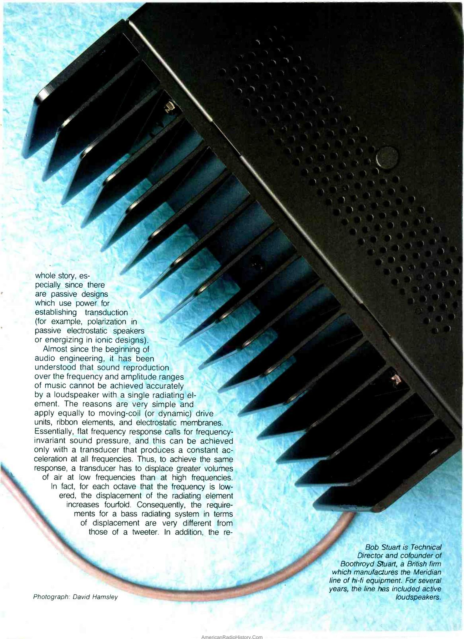
whole story, especially since there are passive designs which use power for establishing transduction (for example, polarization in passive electrostatic speakers or energizing in ionic designs).
