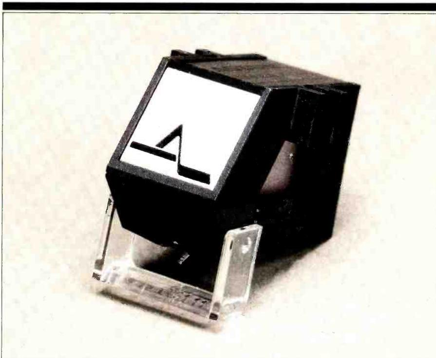
**Output:** 3.5 mV at 5 cm/S at 1 kHz.**Channel Balance:** Within 1 dB at 1 kHz.**Inductance:** 90 mH.**Load Resistance:** 47 kilohms.**Load Capacitance:** 100 pF.**Cartridge Mass:** 5.5 grams.**Price:** \$100.**Company Address:** P.O. Box 120,
