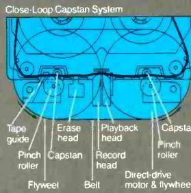
The capstan and flywheel on the take-up side, furthermore, are integral parts of a sophisticated Sony 3-phase linear-torque BSL (brushless/slotless) direct-drive motor with quartz-lock digital servo. In the closed-loop dual capstan configuration, it delivers precise, steady tape travel with remarkably low wow-and-flutter: less than 0.025% (WRMS).
