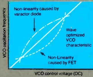
The result in Sony's ST-S700ES tuner is PLL detector that exhibits extremely low distortion and noise.
