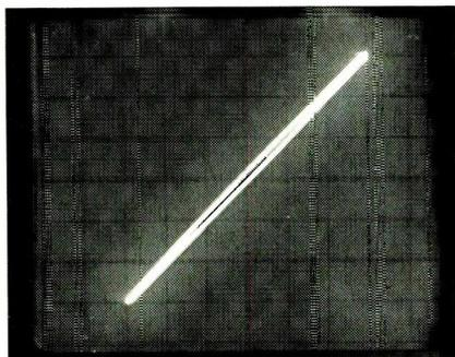
Fig. 8—Interchannel phase comparison at 20 kHz. Slightly elliptical pattern indicates minimal phase error. (See text.)
