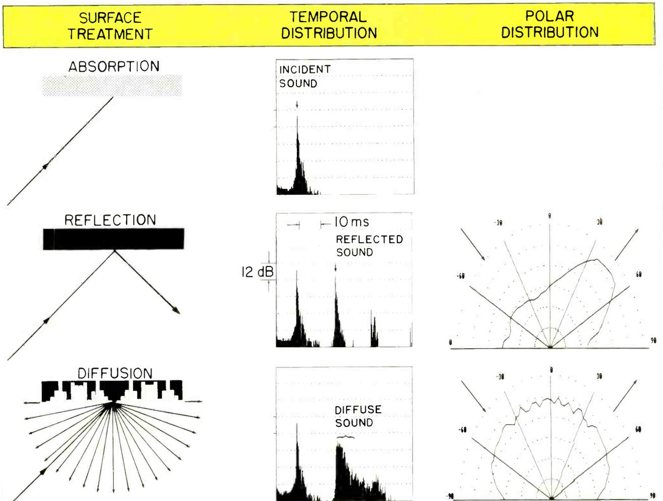
Fig. 2—Comparison of temporal (time) and spatial (polar) diffusing properties of absorptive, reflective, and diffusive surfaces. The scattered energy from an ideal absorptive surface (top row) is negligible; therefore, no polar plot is depicted. The energy scattered from a reflective surface
