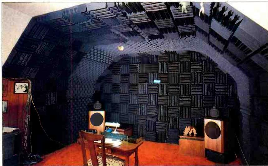
Fig. 6—The dead end of a Live End/Dead End (LEDE) room in Pisha's home. Front speakers are B & W 801Fs and Janis W1 subwoofers.
