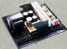
molded at high temperature into a single piece, onto which the power transformer, heat sink and PC board assemblies are mounted. The structure is approximately 3,000 times more rigid than a conventional steel chassis.
