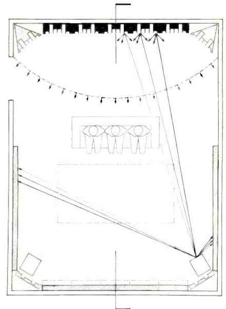
*Fig. 5B—Side view of same room as in Fig. 5A, showing absorption on side walls, vertical Abffusors from floor to ceiling in front corners, and absorptive treatment on ceiling. For greater spaciousness, a diffusive ceiling can be used, in which case upper side walls reflect laterally diffused sound (dashed line with arrow) from ceiling diffusers.*
