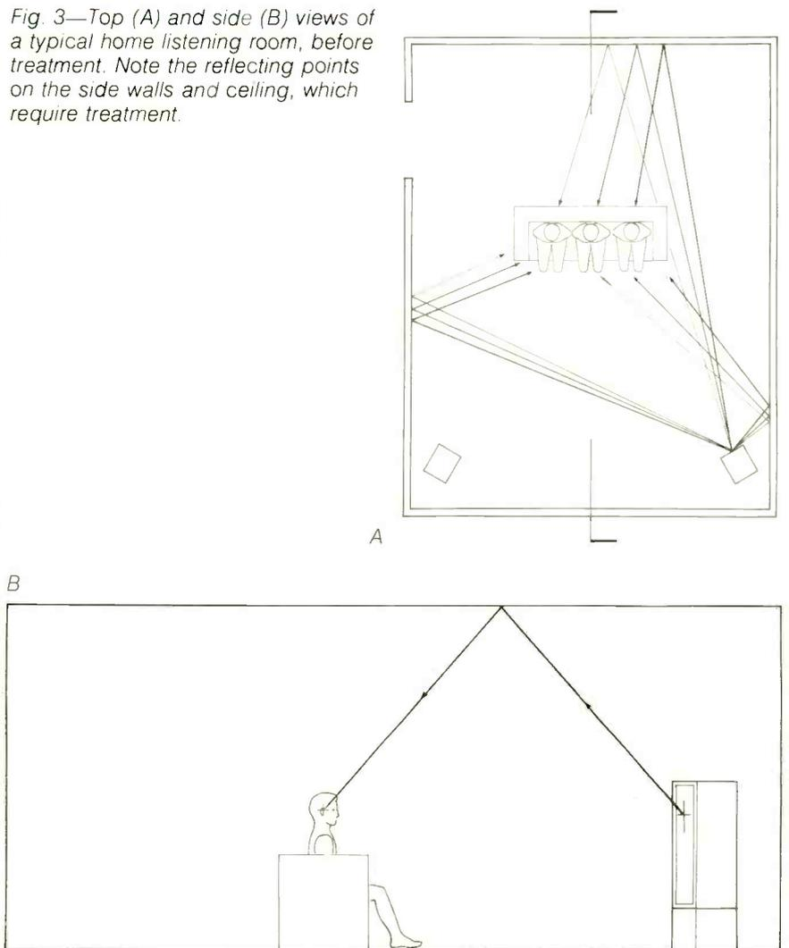
Therefore, to minimize reflections at a listening position, we can make boundary surfaces diffusive or absorptive; alternatively, we can angle and splay speaker boundary surfaces so reflected energy can be directed away from the listening position.
