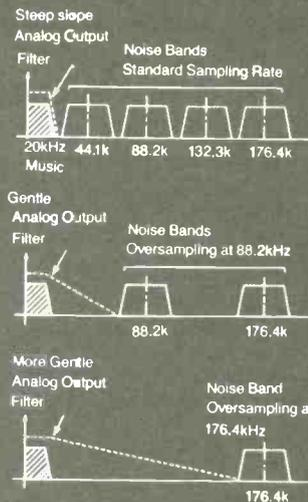
While digital filtering does solve the problems associated with steep analog filters, the interaction of multiple clock rates found in typical oversampling designs creates high-frequency spurious noise. ES Series CD players are free of such noise thanks to Sony's exclusive UniLinear Converter™, which utilizes a single "master clock" to synchronize all digital decoding functions.
