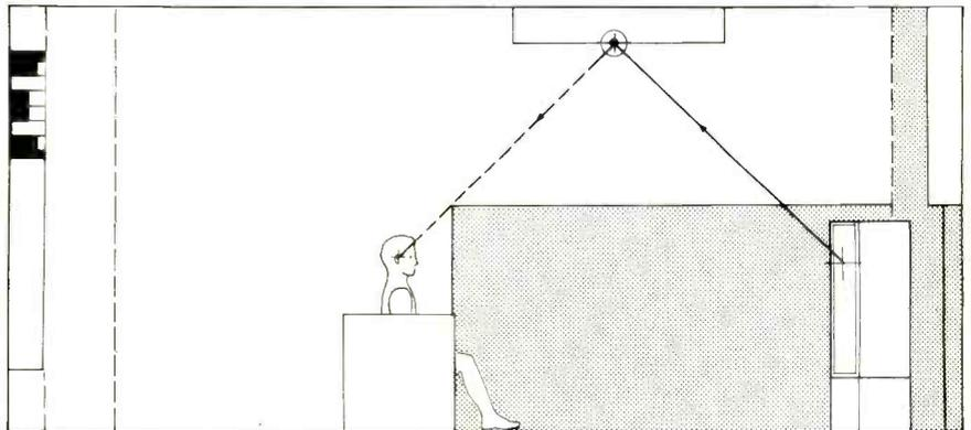
4. Reduce backscattered energy, to minimize interference with the direct sound, frequency coloration, and image shifting.
