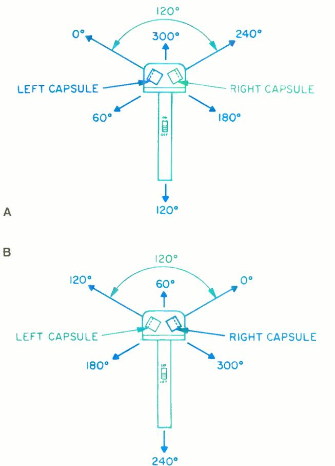
**Fig. 1—Capsule layout of the AT-9400. The angles for the left capsule (A) correspond to the response curves shown in Figs. 3 and 5; angles for the right capsule (B) are for use with Figs. 4 and 6.**
