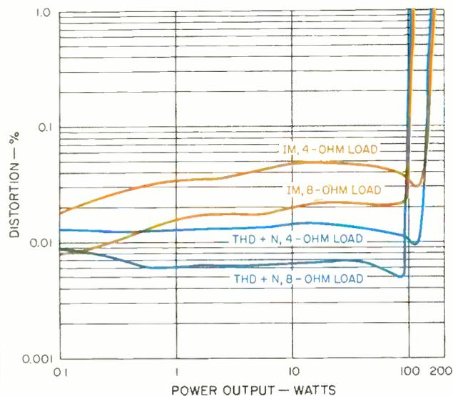
Fig. 2—THD + N at 1 kHz, and SMPTE IM, both vs. power output.
