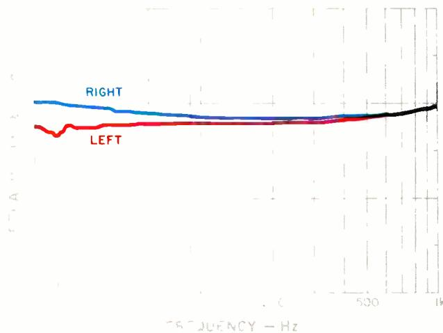
**Fig. 5—**Slow sweep from 20 Hz to 1 kHz. Note absence of "glitches" (see text).
