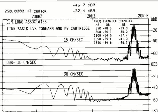
**Fig. 14—Spectrum analysis of output from signals shown in Fig. 13. Distortion is 2.4% at 250 Hz for the 30-cm/S level (bottom trace).**
