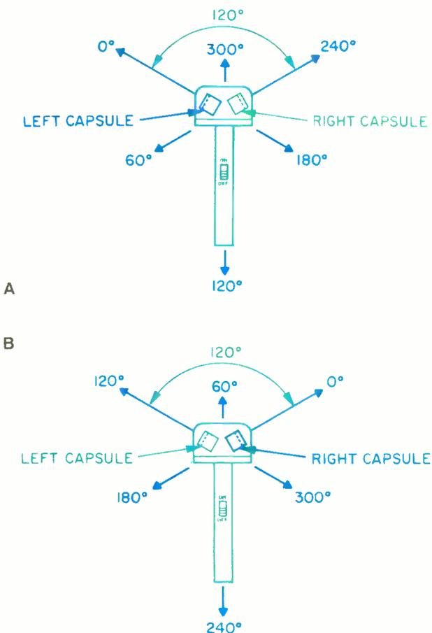
**Fig. 1—Capsule layout of the AT-9400. The angles for the left capsule (A) correspond to the response curves shown in Figs. 3 and 5; angles for the right capsule (B) are for use with Figs. 4 and 6.**
