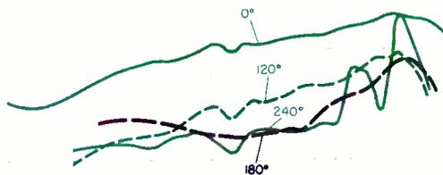
Fig. 6—Same as Fig. 5 but for the right capsule. Here, the 120° curve coincides with the axis of the left capsule, 240° is to the rear of the microphone handle, and 180° is directly behind the capsule.
