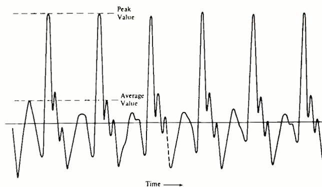
Fig 2—Trumpet waveform (about 400 Hz), with peak-to-average ratio of 13 dB. Signals like this are common in pop-music recordings in which microphones are placed close to
