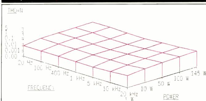
**Fig. 2—THD + N vs. power and frequency, 8-ohm load. Note that THD scale is logarithmic.**
