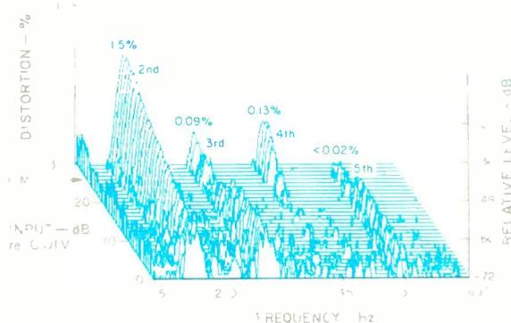
**Fig. 8—Harmonic distortion for the musical tone A<sub>2</sub> (110 Hz).**
