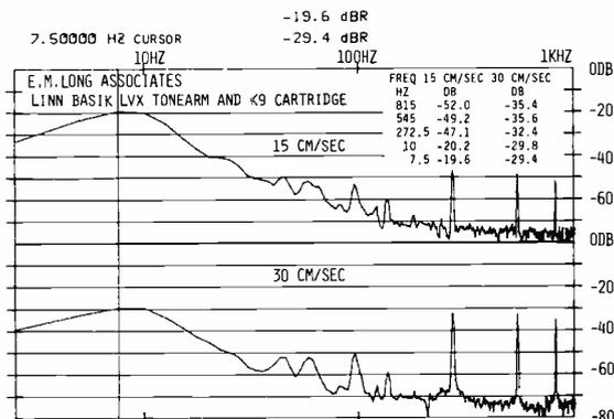
**Fig. 15—Spectrum analysis of distortion products from signals shown in Fig. 13. Note that the frequency range shown runs only to 1 kHz and that the level at the arm/cartridge resonance drops when the signal level is raised (see text).**
