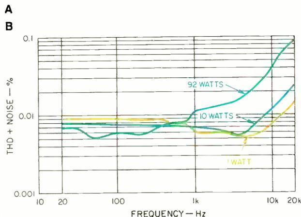
Fig. 1—THD + N vs. frequency for 4-ohm (A) and 8-ohm (B) loads.
