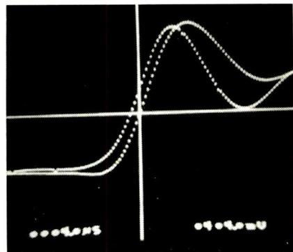
**Fig. 10—Time delay between right and left channels. Right channel leads left by 4.0 μS.**
