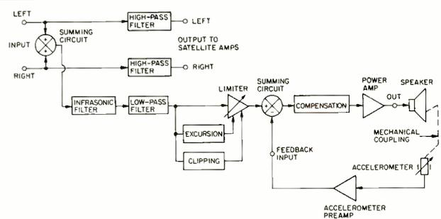
Fig. 1—Block diagram of the ULD-15 (see text).
