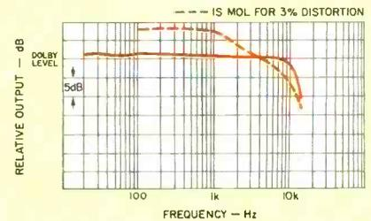
respects. The best-performing Type I tapes, with 400-Hz MOLs of +6 dB or more, match the S/N ratios of many Type II tapes. The Type I overall ratings do not go much beyond 60% at this time because their performance (except for consistency) cannot match that of Type IV tapes.
