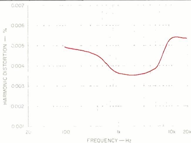
Fig. 1—THD vs. frequency, high-level inputs.
