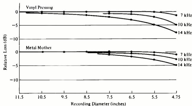
Fig. 4—Change in disc high-frequency response from outer to inner grooves. Signals were recorded at 15 dB below 1-kHz reference velocity of 5.5 cm/s, using RIAA pre-emphasis and de-emphasis curves; playback measurements were made
