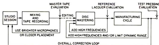
Fig. 5—Corrective feedback processes performed by recording engineers in LP recording and manufacture.
