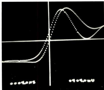
**Fig. 10—Time delay between right and left channels. Right channel leads left by 4.0  $\mu$ S.**
