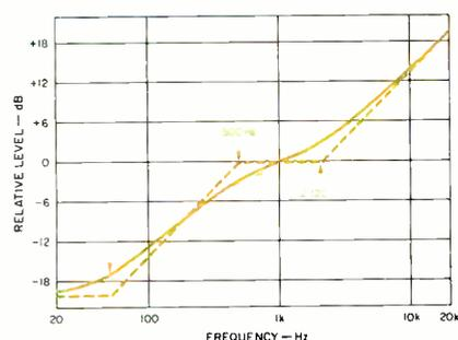
Fig 3—The RIAA pre-emphasis curve used in disc recording to conserve modulation space at low frequencies and raise high frequencies above the inherent disc noise. A complementary de-emphasis curve is used in playback to restore flat response.
