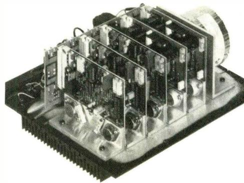
The Plus Beta contains three discrete power amps with digitally controlled active filters. They are frequency-driven and provide dynamic soft clipping for overload protection. The bass amplifier is rated at 100 watts RMS power; the satellite amps at 80 watts RMS per channel. THD is less than 0.01%.
