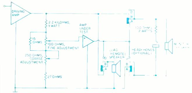
**Fig. 1—Schematic of Hafler's XL-10 test fixture. ("straight wire") output, Switch position A is for listening to the output of the test amplifier, position B for bypassing to hear the driving amp's direct**
