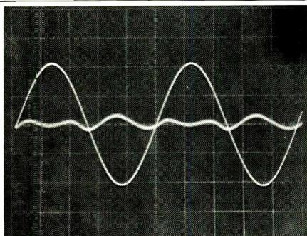
Fig. 3—THD at 1 kHz for 10 watts output into 8-ohm load. Large trace is output signal; small trace is distortion residue after subtracting input frequency.
