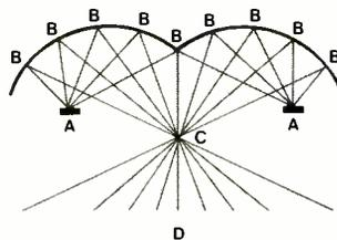
Sound from two matched 1" tweeters (A) is directed at the Ferralipse Acoustic Lens. Highs are then reflected (B) to a central focal point (C), which radiates through a 120° horizontal angle (D) with far greater uniformity and efficiency than traditional designs.
