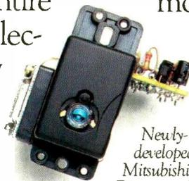
*Newly-developed Mitsubishi Photo-Direct amplifier maintains signal integrity by combining the photodiode detector and preamplifier at the pickup.*
