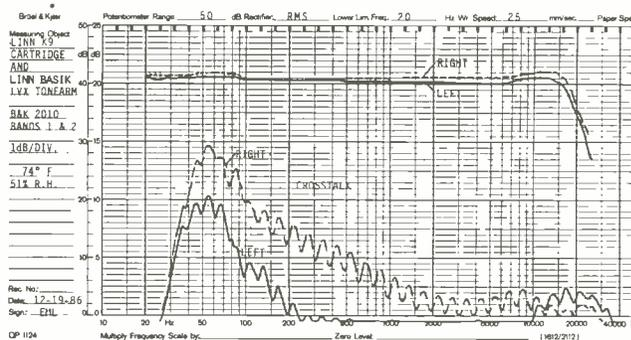
**Fig. 1—Frequency response and crosstalk, K9 cartridge in Basik LVX arm, using B & K 2010 test record.**
