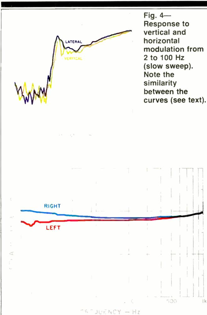
**Fig. 4—**Response to vertical and horizontal modulation from 2 to 100 Hz (slow sweep). Note the similarity between the curves (see text).
