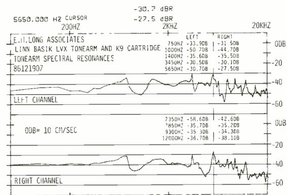
**Fig. 7—Spectral output of arm/cartridge for mechanical impulses applied to armtube; traces shown are average of 16 impulses.**
