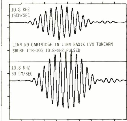
**Fig. 13—Response to 10.8-kHz pulse, Shure TTR-103 test record.**
