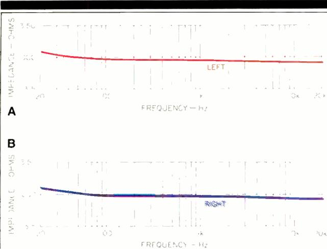
**Fig. 2—Impedance of left (A) and right (B) capsules. The two curves are virtually identical, and impedance (920 ohms at 1 kHz) is lower than the rated 1.5 kilohms. Note that impedance scale is logarithmic.**
