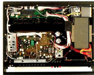
A glimpse inside reveals how carefully thought-out the R4 is. No space is wasted. Electronic circuitry, heat sinks, transformers, etc., are all contained within a box that stands only 2¾" high.
