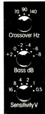
The Plus Beta's control panel allows adjustment of: crossover point, for perfect matching with any satellite loudspeakers; input sensitivity, to optimize preamp compatibility; and bass level control to adapt for room characteristics.
