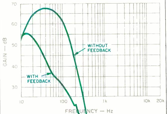
Fig. 2—Amplifier frequency response, measured from left input to speaker terminals, with feedback loop both connected and opened.
