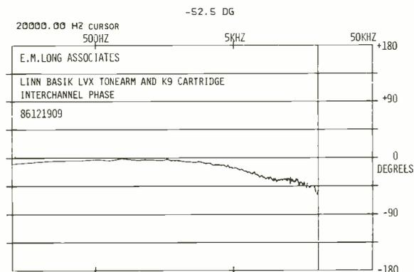
**Fig. 9—Interchannel phase difference vs. frequency from B & K 2011, band 7, pink noise.**
