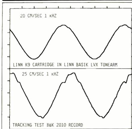
**Fig. 11—Tracking test of K9 cartridge in Basik LVX arm shows very little jitter, which indicates good stability. The mistracking in the lower graph is with the highest level band of B & K 2010; the performance is quite good.**
