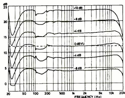
Fig 1—Analog-tape output curves for six recording levels. Note how high-frequency roll-off above 8 kHz increases with recording level. Recordings were made at 15 ips; kink in curves between 100 and 200 Hz is an artifact of the measuring system. (Data taken from John Borwick, *Sound Recording Practice*, Oxford University Press, London, 1976, pg. 119.)
