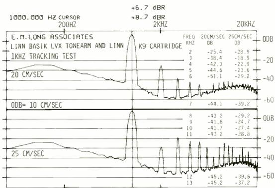
**Fig. 12—Spectrum analysis of the cartridge output when reproducing the test tones of Fig. 11. The third harmonic (at the**
