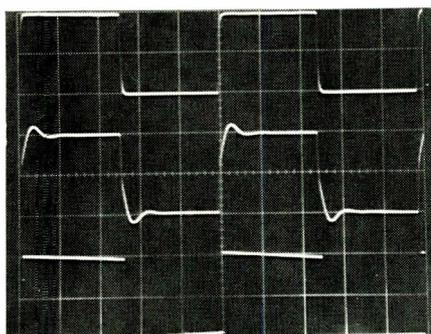
Fig. 4—Square-wave response for 10 kHz into 8-ohm load (top), 10 kHz into 8 ohms paralleled by 2  $\mu$ F (middle), and 40 Hz into 8 ohms (bottom). Scales: Vertical, 5 V/cm; horizontal, 20  $\mu$ S/cm (top and middle), 5 mS/cm (bottom).
