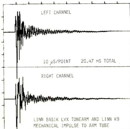
**Fig. 6—**Output vs. time of arm/cartridge when mechanical impulse was applied to arm tube, with arm on rest but not clamped.
