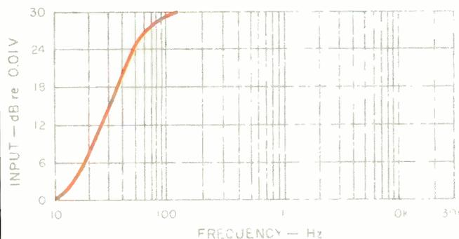
**Fig. 9—Limiter action. Input voltage needed to cause a given level of compression varies with frequency to limit cone**
