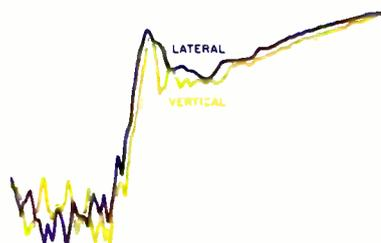
**Fig. 4—**Response to vertical and horizontal modulation from 2 to 100 Hz (slow sweep). Note the similarity between the curves (see text).
