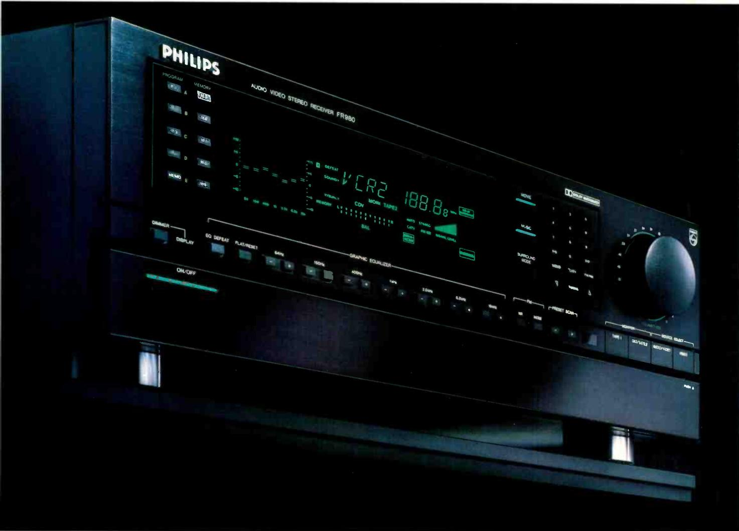
Motorized main analog volume control. Digitally synthesized AM/FM stereo tuner with 19 presets. 7-band graphic equalizer with Acoustic Memory feature. Record out selector allows separate recording and listening. Video and audio dubbing capability. Cable FM/TV ready. Pre-out and main-in connections.
