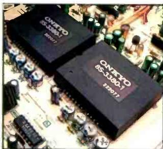
Most of our models also benefit from Opto-Coupling, an Onkyo-developed technology that transmits data optically rather than through conventional wiring for more accurate CD sound.
