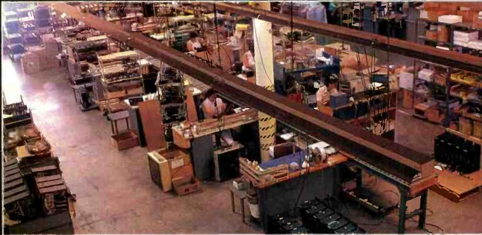
One hundred percent quality control is seen on EVERY unit manufactured. EVERY completed unit is electronically tested for specification accuracy and then EVERY unit is connected to a high fidelity system and listened to—just like you would at home. If your unit meets or exceeds the critical standards set forth on these tests, it is then packaged for shipment.
