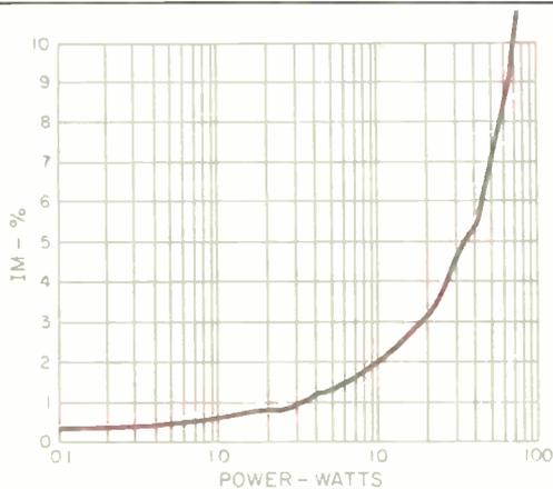
**Fig. 11—IM distortion on 440 Hz (A<sub>4</sub>) produced by 41.2 Hz (E<sub>1</sub>) when mixed in one-to-one proportion.**
