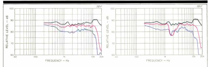
Fig. 8—Mean horizontal on- and off-axis frequency response curves above 200 Hz; see text. Top curve is mean on-axis curve, an average of response measurements made within  $\pm 15^{\circ}$  of vertical and horizontal axes. Middle curve is average of measurements between 30° and 45° either side of axis; bottom curve is average of measurements 60° to 75° either side of axis. Note the very smooth off-axis response, even at angles out to  $\pm$ 75°.
