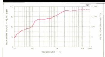
Fig. 18—Maximum peak-input power for moderately clean output. Above about 6 kHz (dashed portion of curve), limitations are imposed by clipping of 5.5-kilowatt amplifier, not by the speaker. Input signal was a shaped tone burst; see text.
