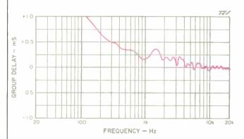
Fig. 3—Group delay corresponding to phase response of Fig. 2. The woofer lags the tweeter by about 0.17 mS, an equivalent distance of 2.3 inches.
