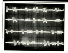
Fig. 7—Surround outputs for modified version of "Symphony Hall 5" preset program, with 2-cycle, 300-Hz tone burst fed to input. Results shown are, from top to bottom, for left F/DAP output, right F/DAP output, left R/DAP output, and right R/DAP output.
