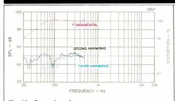
Fig. 16—Second- and third-harmonic distortion levels vs. frequency for 90 dB SPL mid-band output at 1 meter on axis; input signal is 3.6 V rms (1.6 watts into 8 ohms).
