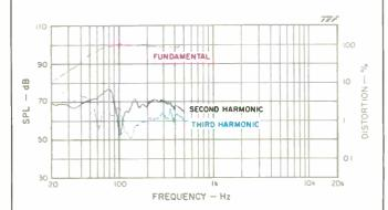
Fig. 17—Same as Fig. 16 but for 100 dB SPL mid-band output, using input signal of 11.3 V rms (16 watts into 8 ohms).
