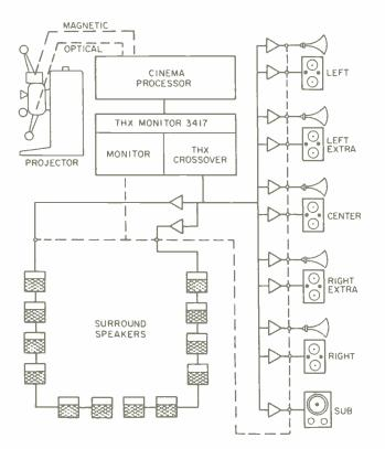
Fig. 1—Block diagram of typical 70/35-mm THX Sound System. Theaters using only 35 mm do not require the "Left Extra" and "Right Extra" screen speakers.
