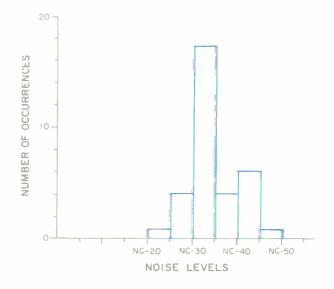
Fig. 7—Statistical distribution of background-noise levels in typical theaters. Nost of the theaters in this survey, made by the Theater Alignment Program for the National Association of Theater Owners, would not qualify for THX certification without modifications.
