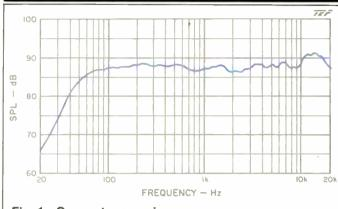
Fig. 1—One-meter on-axis frequency response, with an input of 2.83 V rms (equivalent to 1 watt into the rated 8-ohm impedance).
