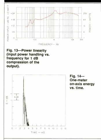
Power linearity, plotted for the Ensemble in Fig. 13, is a full-range test of power handling. Power is increased at each frequency, until the acoustic output fails to increase along with it. The Ensemble accepts only moderate power in the bass, but it is linear in most of the upper range, with the maximum 256-watt input I use for these tests. It is evident that using amps with more than 150 watts output would be of little benefit with the Ensemble.
