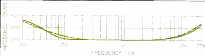
**Fig. 1—Output impedance vs. frequency with response switch set for “flat” (solid curve) and low-cut (dashed curve).**
