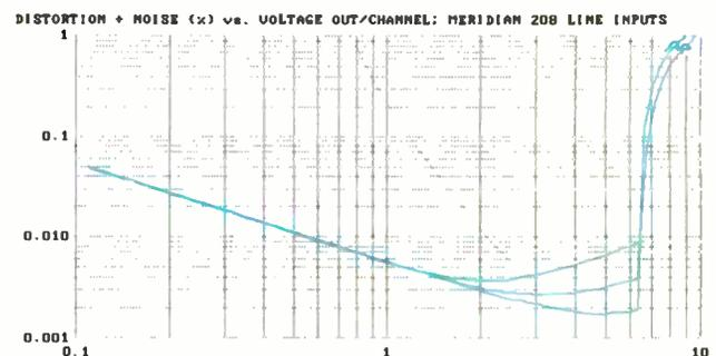
Fig. 12—THD + N vs. output voltage for preamp section line inputs and outputs. Curves are, top to bottom, for 20 kHz, 1 kHz, and 20 Hz.
