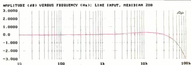
Fig. 11—Frequency response of preamp section, using line inputs.
