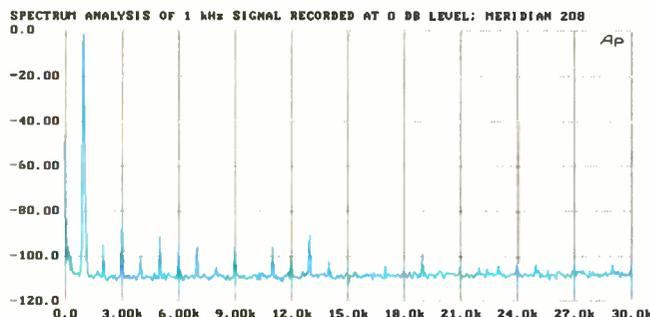
**Fig. 4—Spectrum analysis of 1-kHz signal at 0 dB recorded level.**
