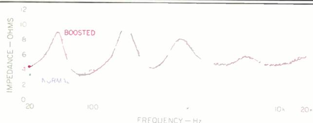
**Fig. 1—Impedance vs. frequency.** The "Normal" curve is with "Bass Roll-Off" set at "1" and all other straps at "0 dB"; the "Boosted" curve is with "Bass Roll-Off" at "2" and all other straps at "+1 dB," the setting which produces the most difficult load.
