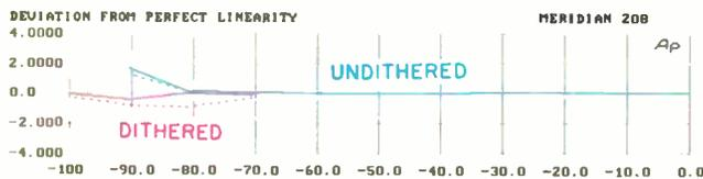
Fig. 9—Deviation from perfect linearity, for dithered and undithered signals.
