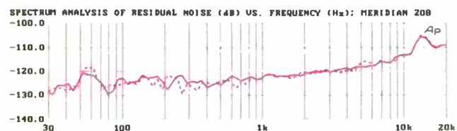
Fig. 7—Spectrum analysis of residual noise when playing "no signal" test track.
