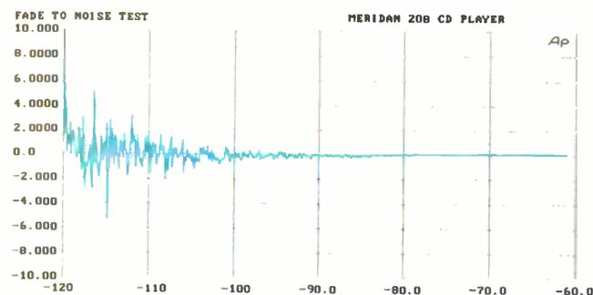
Fig. 10—Fade-to-noise test, using dithered signals from -10 to -60 dB.
