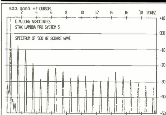
Fig. 4—Spectrum of the 500-Hz square wave as reproduced by the Stax headphones. The output is a little high at 2.5 kHz, low at 4.5 kHz, and high above 13.5 kHz.
