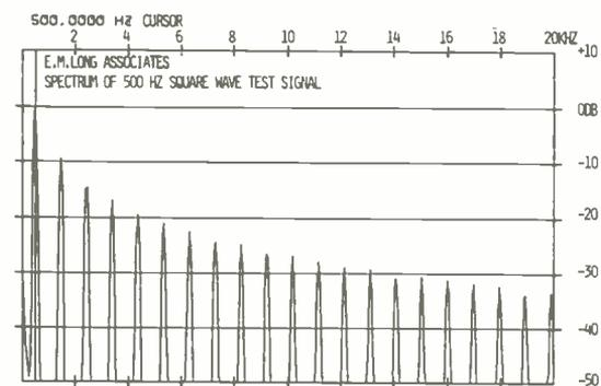
Fig. 3—Spectrum of the 500-Hz square wave shown in Fig. 2, for reference use. The harmonics are spaced at 1-kHz intervals across the spectrum.
