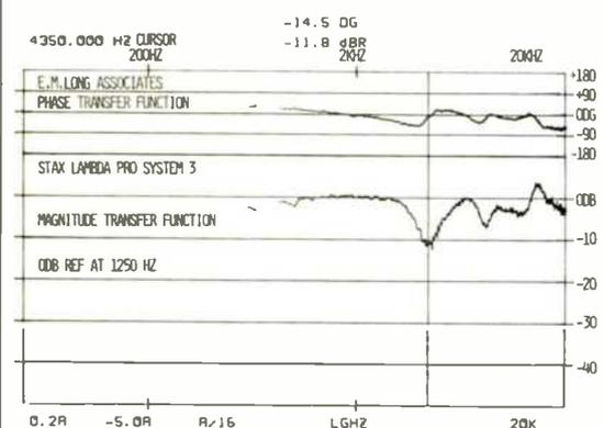
Fig. 6—Phase and amplitude spectra produced by the SR-Lambda Pro for the 30-kHz cosine pulse shown in Fig. 5. This and other curves are meant as relative measurements only, for comparison with curves in future reports. They are not meant as absolute measurements; see text.
