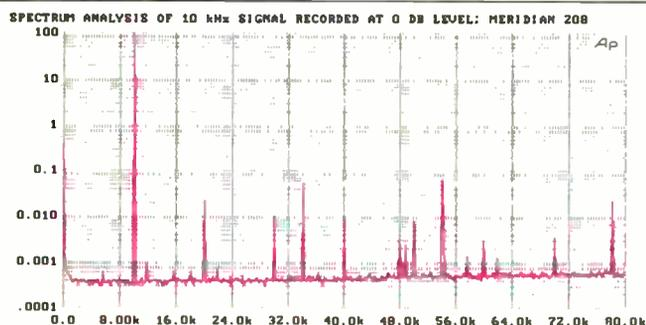
Fig. 5—Spectrum analysis of 10-kHz signal at 0 dB recorded level.
