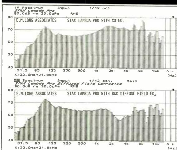
Fig. 1—Stax SR-Lambda Pro headphones as measured by B & K HATS Manikin, without and with B & K diffuse-field equalization; the bump in response at about 100 Hz is due to incomplete sealing of the earcushions on the artificial head. The equalization provided by B & K is greater than necessary for these phones; see text.
