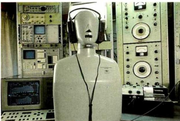
Fig. 5—Brüel & Kjaer Head and Torso Simulator (HATS), with headphones in place.
