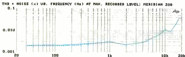
**Fig. 2—THD + N vs. frequency.** Rise in curve at high frequencies is actually due to out-of-band beats, not increased THD.
