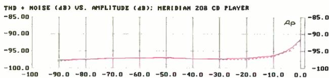
**Fig. 3—THD + N vs. level for a 1-kHz tone.**
