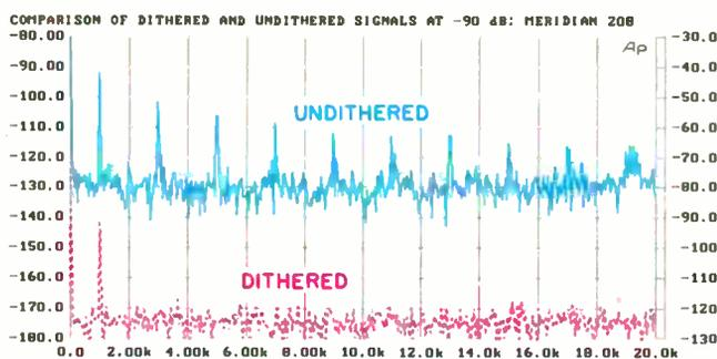
Fig. 6—Spectrum analysis of 1-kHz signals at -90 dB recorded level. Use left-hand scale for upper curve, right-hand scale for lower curve.
