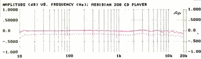
**Fig. 1—Frequency response.** Left channel is shown by solid curve and right channel by dashed curve in this and subsequent figures, except where noted.
