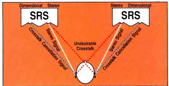
*Each Polk SDA incorporates a special extra set of drivers which radiate a difference signal that cancels the undesirable signal going from the wrong speaker to the wrong ear (interaural crosstalk distortion).
