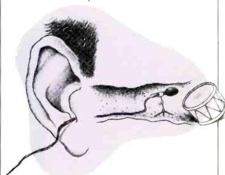
He used newly developed wide-range miniature microphones designed to be placed in the ear canal, almost touching the eardrum. Listeners with such microphones in their ears were then exposed to acoustic test signals from speakers and the frequency response and energy-time curve (ETC) were recorded. Breithaupt found significant frequency response differences between individuals for different sound-source positions in the horizontal plane.
