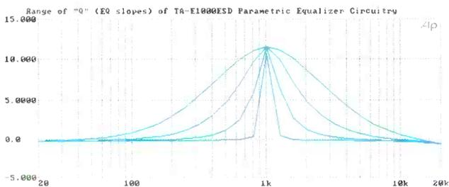
**Fig. 4—Range of slopes that can be assigned to any of the three parametric equalizer bands, at maximum boost setting. Slopes for maximum cut setting were identical.**
