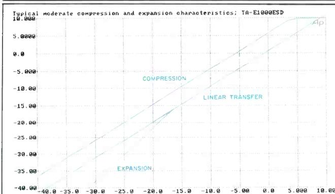
**Fig. 5—Typical compression and expansion characteristics of Sony TA-E1000ESD, superimposed on linear transfer curve. Input levels are shown on horizontal axis, output levels on vertical axis; see text.**
