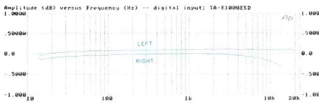
**Fig. 1—Frequency response at analog outputs, for right-channel line-level analog input (A) and for left- and right-channel digital input (B).**
