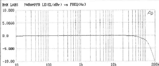
**Fig. 1—**Frequency response for 8-ohm loads on the 8-ohm taps.
