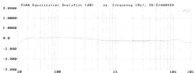
**Fig. 2—Deviation from RIAA equalization.**
