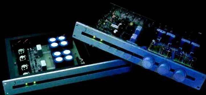
The DMC-20 establishes a benchmark in preamplifier design. Spectral's innovative architecture provides seven audio sources, phase switching, and full tape facilities. The DMC-20 can provide precise loading for any phono cartridge. It can offer fully differential balanced input and output capability.
