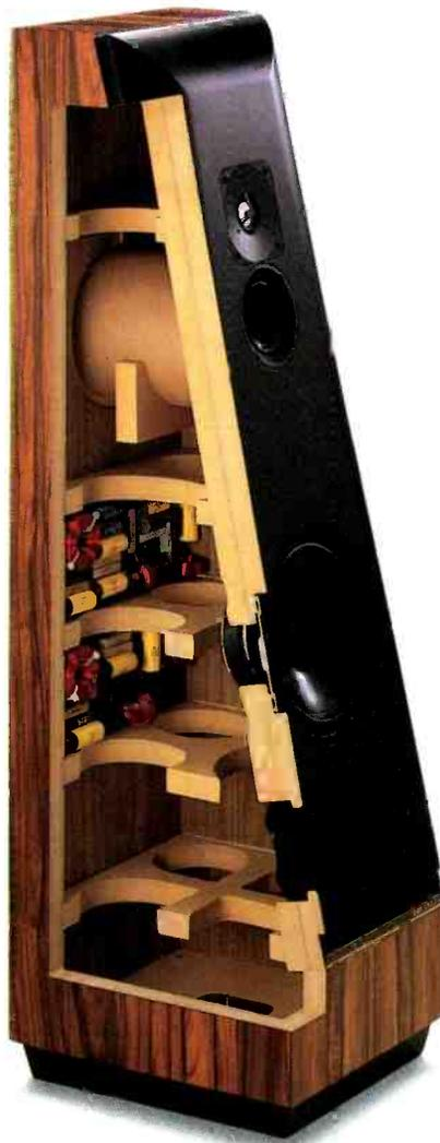
The same 1" metal dome tweeter used in the model CS5 eliminates resonances, energy storage and colorations in the audible range. The short coil/long gap, large suspension design provides very low distortion and high dynamic range. The result is high frequency reproduction of unparalleled clarity and realism.
