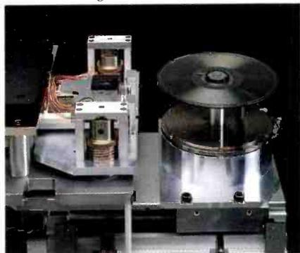
The OMS-2000's optical transport mechanism provides absolute positioning with unrivaled precision.
