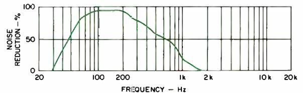
Anti-noise bus muffler (courtesy of NCT)
