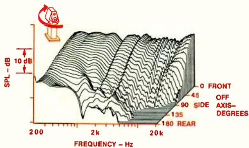
Fig. 4—Horizontal off-axis frequency responses.
