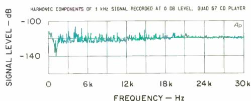
Fig. 3—Spectrum analysis of harmonics of 1-kHz, 0-dB signal.
