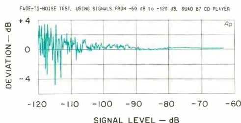
**Fig. 7—Fade-to-noise test.**
