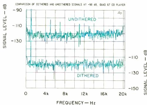
**Fig. 5—Spectrum analysis of 1-kHz signals at -90 dB. (Use right-hand scale for "Dithered" curve.)**
