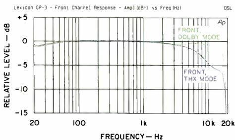
**Fig. 2—Front-channel response, processed modes.**
