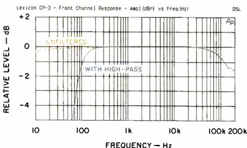
**Fig. 1—Front-channel response, unprocessed mode. Note expanded scale.**
