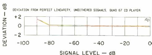
**Fig. 6—Deviation from perfect linearity, undithered signals.**
