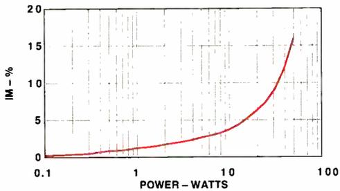
Fig. 12—IM distortion for  $A_4$  (440 Hz) and  $E_1$  (41.2 Hz).
