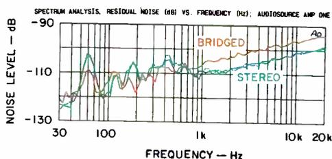
Fig. 7—Spectrum analysis of residual noise.
