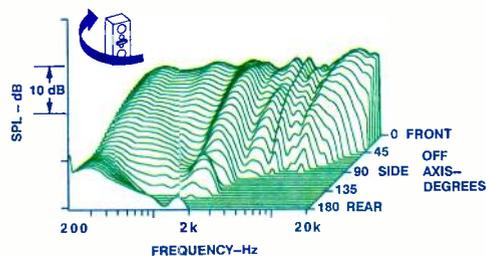
Fig. 4—Satellite horizontal off-axis frequency responses.
