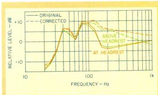
**Fig. 3**—Response of car sound system with original, factory-inverted polarity and with polarity corrected.
