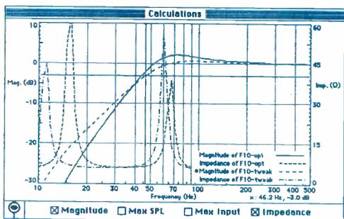
**Fig. 1—Impedance and response curves, Macintosh version.**
