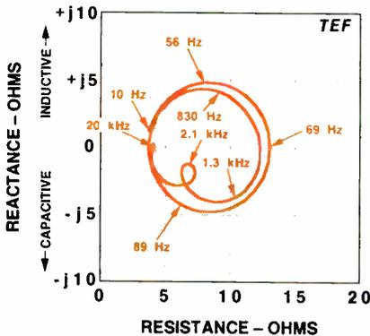
Fig. 7—Satellite complex impedance.
