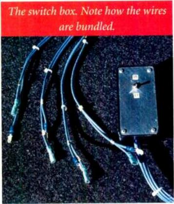
To install the switch, connect the L.AMP+ wire from the switch to a wire from the left-channel amplifier, and the L.SPKR+ wire to the left-speaker wire with the same color as L.AMP+, as was shown in Fig. 4. Connect both the L.AMP- and the L.SPKR- wires as above, then the
