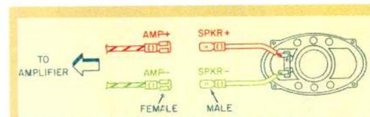
**Fig. 5**—Connectors added to speaker wires.
