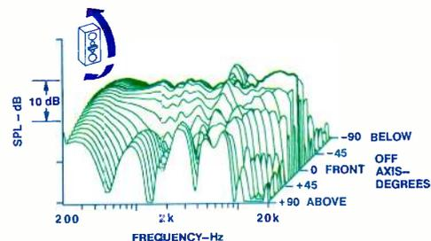
Fig. 5—Satellite vertical off-axis frequency responses.
