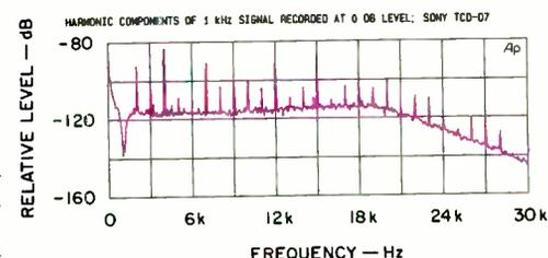
Fig. 4—Harmonics of 1-kHz, 0-dB signal.
