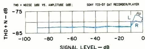
Fig. 3—THD + N vs. signal level.
