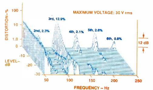
**Fig. 11—Harmonic distortion for E<sub>1</sub> (41.2 Hz).**
