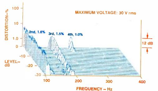
**Fig. 12—Harmonic distortion for B<sub>1</sub> (61.7 Hz).**
