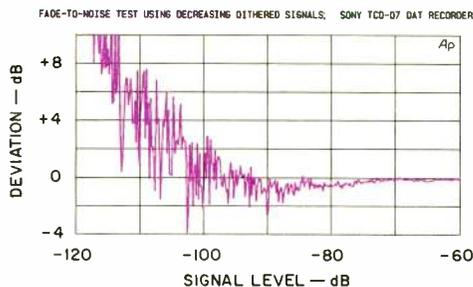
Fig. 8—Fade-to-noise test.
