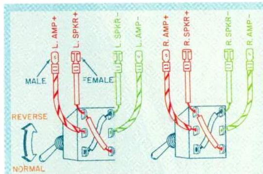
**Fig. 4**—Wiring diagram for the polarity-reversal test-switch setup
