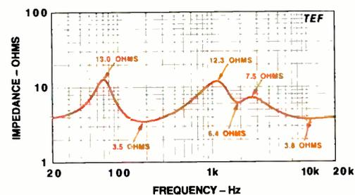
Fig. 6—Satellite impedance.
