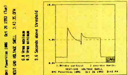
Fig. 2—Neutral-to-ground voltage swell in the a.c. power line over 9.6 seconds. This could increase the line voltage by 5.1 V over the average level.
