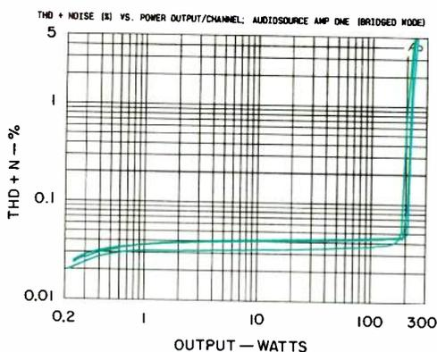
Fig. 6—THD + N vs. power output in bridged mode for three test frequencies; bottom curve is for 20 kHz.
