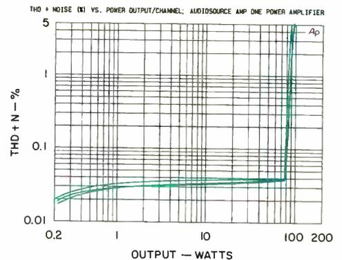
Fig. 3—THD + N vs. power output per channel, for three test frequencies.
