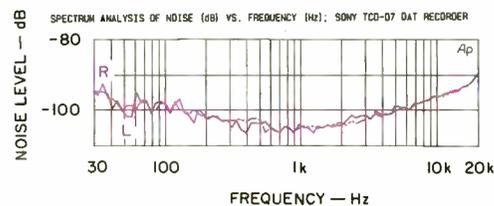
Fig. 6—Spectrum analysis of residual noise from "no-signal" track.
