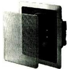
The WS008A is constructed from a one-piece baffle and chassis to reduce vibrations. The woofer has a mineral filled polypropylene cone with a rubber surround and high temperature Kapton voice coil. The tweeter is a 1" Aluminum dome with a Neodymium magnet and ferrofluid cooling. The crossover is 24dB per octave, with polypropylene capacitors in the tweeter circuit for greater clarity.
