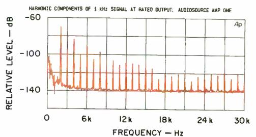
Fig. 4—Spectrum analysis of 1-kHz signal at rated output.
