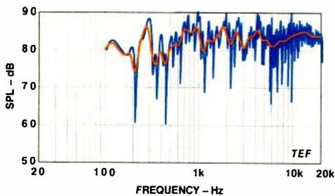
Fig. 8—Satellite 3-meter room response.
