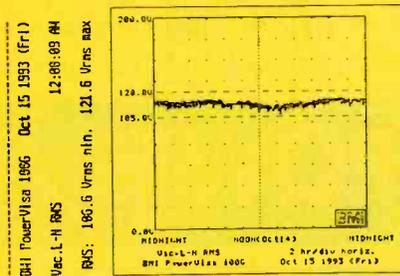
Fig. 1—Variation in the a.c. power line's voltage over a 24-hour period. The variation is 15 V, from 106.6 to 121.6 V.
