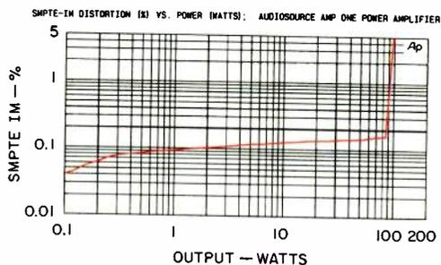
Fig. 5—SMPTE-IM distortion vs. power output, for 8-ohm loads.
