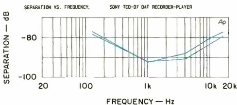
Fig. 5—Separation vs. frequency.
