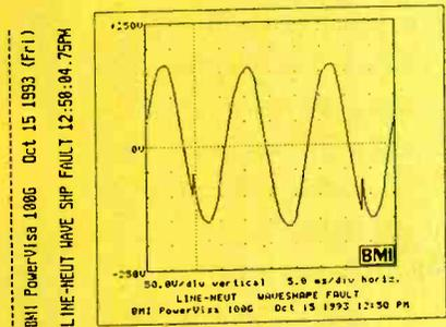
Fig. 4—Distortion of the a.c. power line's sine wave. The glitches in the waveform produce a series of harmonics.
