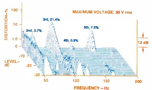
**Fig. 10—Subwoofer harmonic distortion for C<sub>1</sub> (32.7 Hz).**
