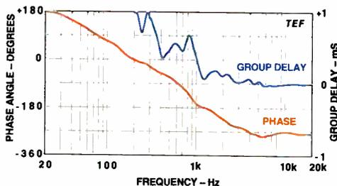
**Fig. 2—Satellite phase response and group delay.**
