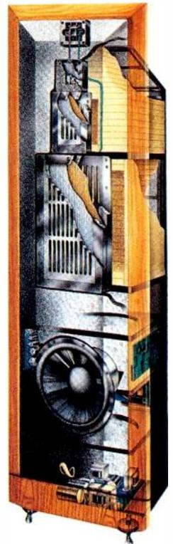
inch thick, and is lined with sound-absorbing material. The planar drivers are also enclosed, to absorb their back waves so as to reduce the comb-filter effects from front-to-rear phase cancellations; Infinity calls this design "radiation pattern control."
