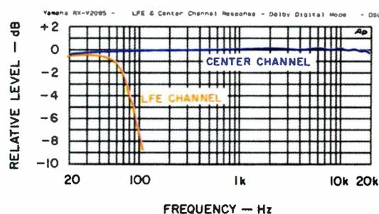
Fig. 13—Frequency response of center and LFE channels, Dolby Digital mode.
