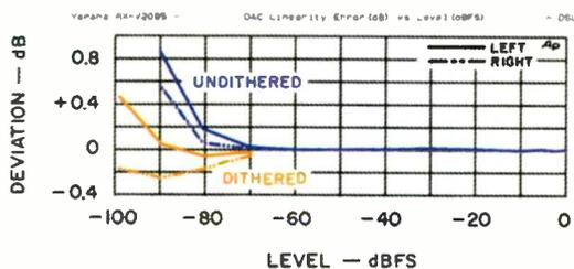
Fig. 10—Linearity error, D/A section.
