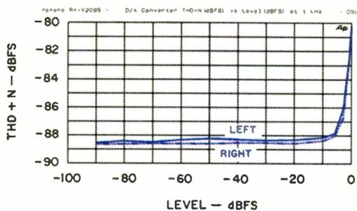
Fig. 9—THD + N vs. level, D/A section.
