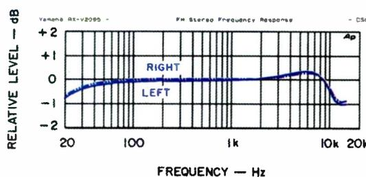
Fig. 15—Frequency response, FM tuner section.
