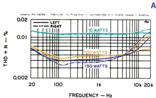
**Fig. 2—THD + N vs. frequency, stereo mode, for 8 ohms (A) and 4 ohms (B).**
