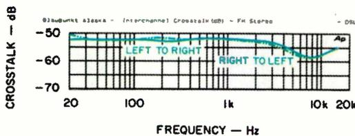
**Fig. 3—Crosstalk, FM tuner section.**
