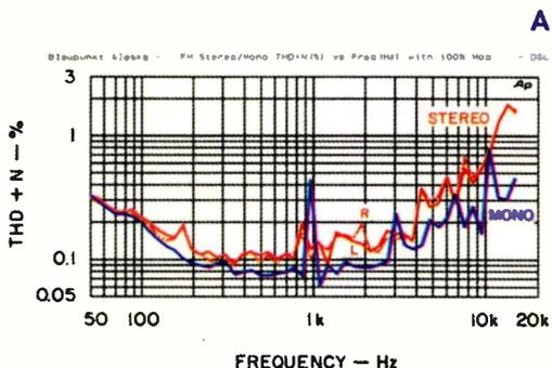
**Fig. 4—THD + N vs. frequency at 50% modulation (A) and at full modulation (B), FM tuner section.**
