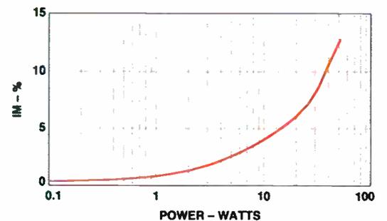
**Fig. 9—IM distortion for A<sub>4</sub> (440 Hz) and E<sub>1</sub> (41.2 Hz).**
