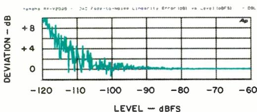
Fig. 11—Fade-to-noise test.
