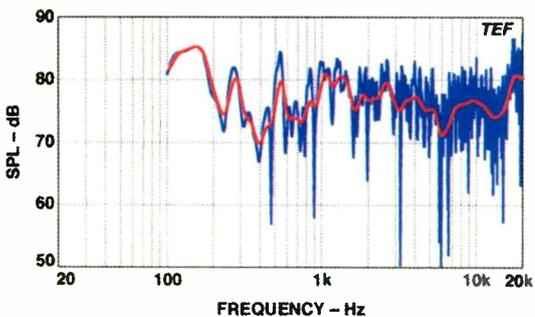
**Fig. 6—Three-meter room response.**
