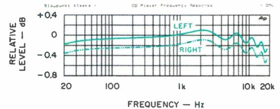
Fig. 6—Frequency response, CD section.
