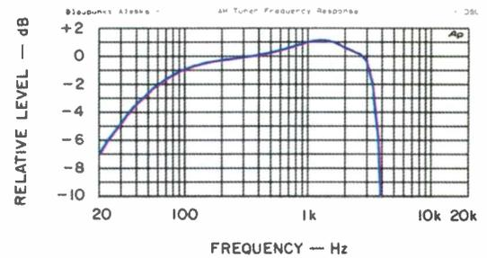
Fig. 5—Frequency response, AM tuner section.
