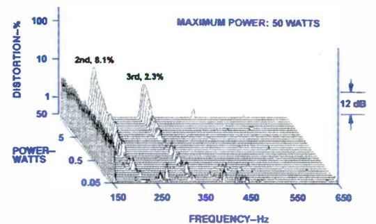
**Fig. 8—Harmonic distortion for  $A_2$  (110 Hz).**
