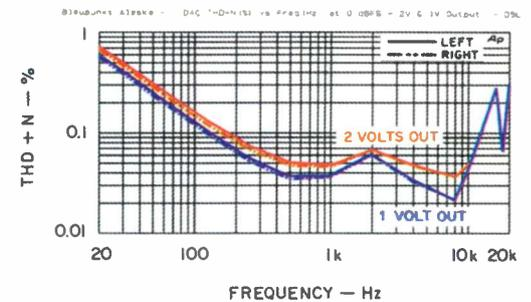
Fig. 7—THD + N vs. frequency, CD section.
