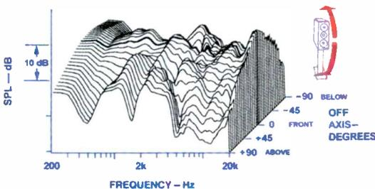
**Fig. 4—Vertical off-axis frequency responses.**
