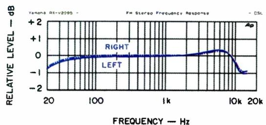
**Fig. 15—Frequency response, FM tuner section.**
