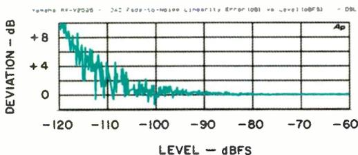
Fig. 11—Fade-to-noise test.
