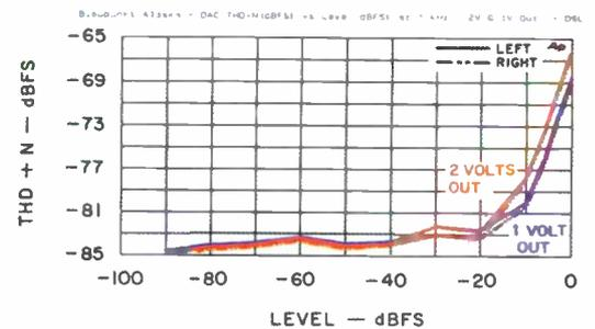
Fig. 8—THD + N vs. level, CD section.
