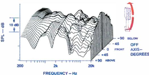
**Fig. 4—Vertical off-axis frequency responses.**
