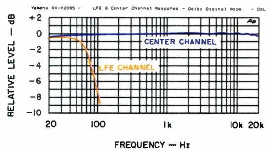
**Fig. 13—Frequency response of center and LFE channels, Dolby Digital mode.**
