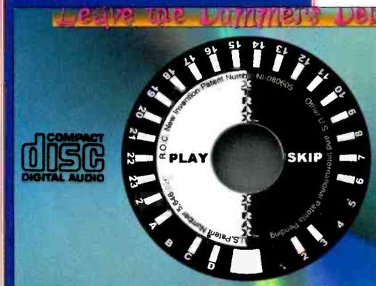
change that. The Xtrax user-preference system consists of CD labels you can mark and unmark as your track choices change plus a label-reading sensor and software to be built into CD players. Cost, says the company, should be negligible.
