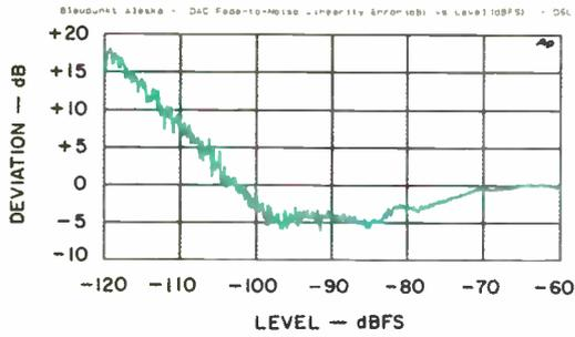
Fig. 10—Fade-to-noise test.
