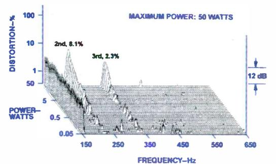
**Fig. 8—Harmonic distortion for A<sub>2</sub> (110 Hz).**
