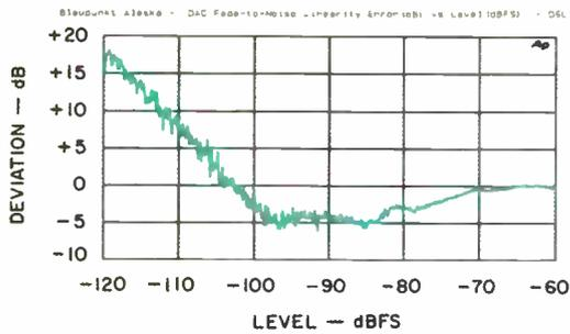
Fig. 10—Fade-to-noise test.
