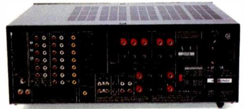
**THE RX-V2095 IS EQUIPPED WITH SIX JACKS TO ACCEPT AN AUDIO FEED FROM AN EXTERNAL DECODER.**
