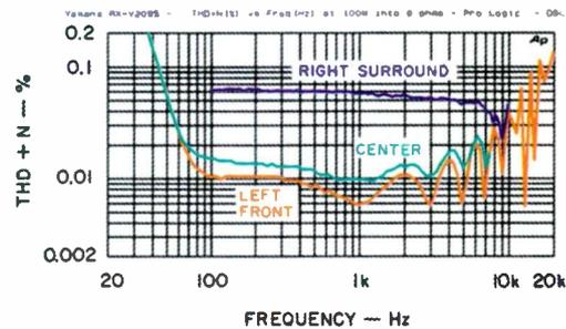
**Fig. 6—THD + N vs. frequency, Dolby Pro Logic mode.**
