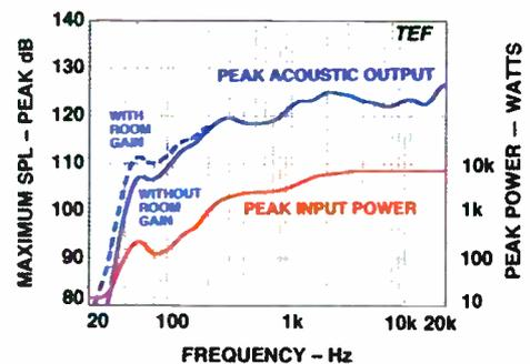
**Fig. 10—Maximum peak input power and sound output.**
