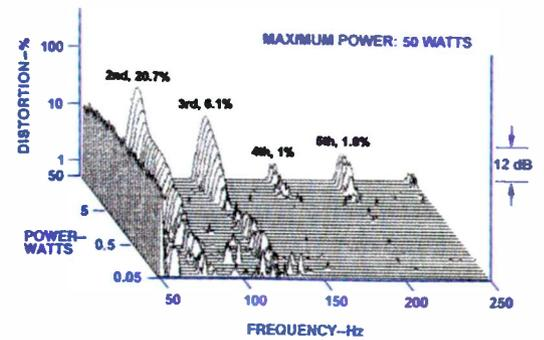
**Fig. 7—Harmonic distortion for  $E_1$  (41.2 Hz).**
