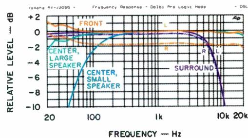
**Fig. 5—Frequency response, Dolby Pro Logic mode.**
