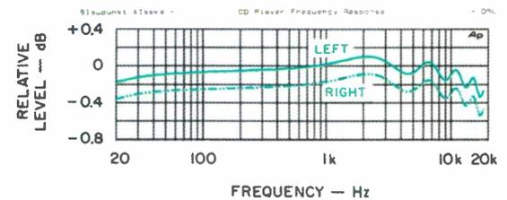
Fig. 6—Frequency response, CD section.
