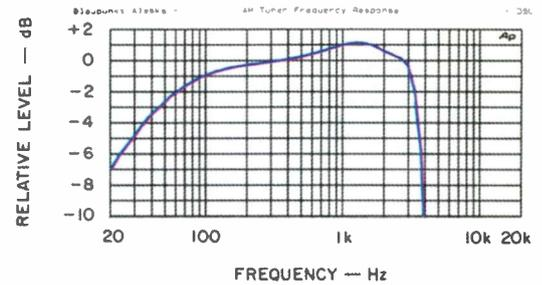
Fig. 5—Frequency response, AM tuner section.
