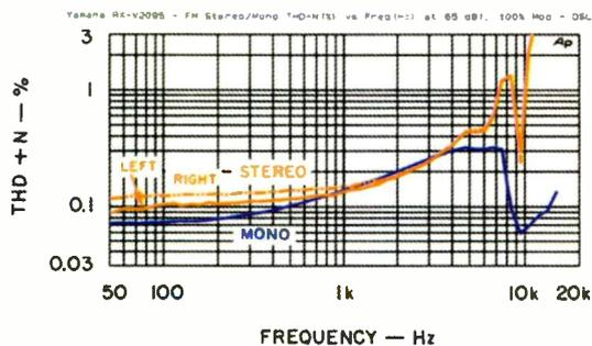
Fig. 17—THD + N vs. frequency, FM tuner section.
