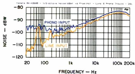
**Fig. 4—Noise analysis, stereo mode.**
