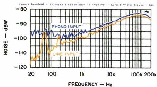
Fig. 4—Noise analysis, stereo mode.
