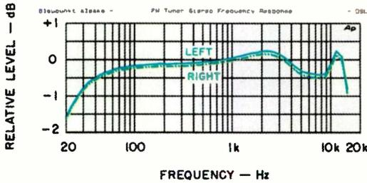
**Fig. 2—Frequency response, FM tuner section.**
