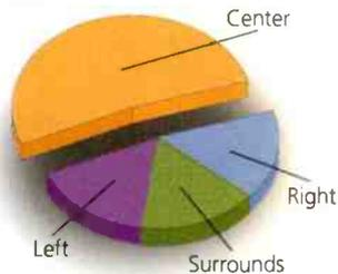
The center channel speaker typically reproduces over 50% of a movie soundtrack’s sound. That means the center speaker must have full dynamic range and high power handling capabilities.
