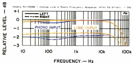
Fig. 3—Frequency response, stereo mode.
