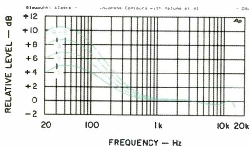
Fig. 13—Loudness compensation with volume adjusted for 30-dB attenuation. At this level, the contours for three of the six compensation settings were the same.
