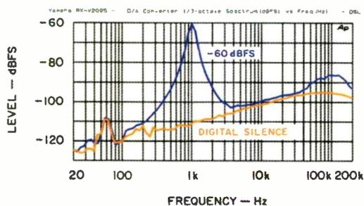
Fig. 12—Noise analysis, D/A section.
