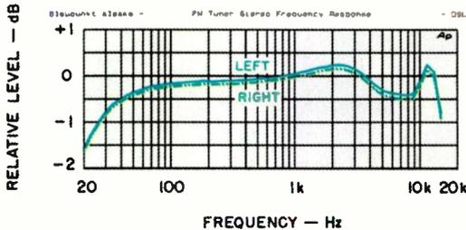
**Fig. 2—Frequency response, FM tuner section.**
