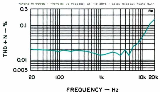
**Fig. 14—THD + N vs. frequency, worst channel, Dolby Digital mode.**
