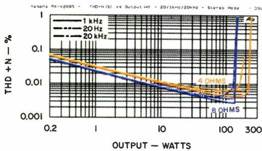
Fig. 1—THD + N vs. output, stereo mode.
