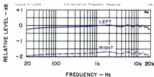
**Fig. 7—Frequency response, D/A section.**
