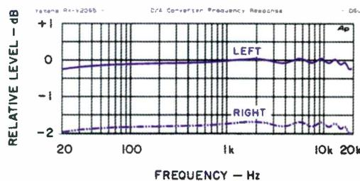
**Fig. 7—Frequency response, D/A section.**
