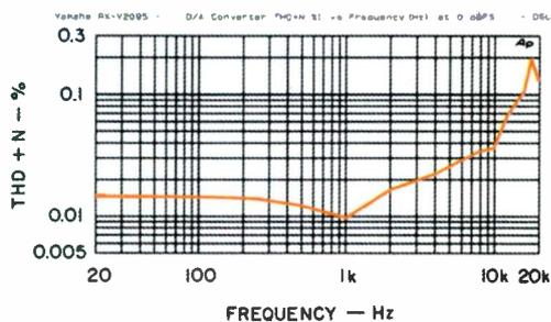
**Fig. 8—THD + N vs. frequency at 0 dBFS, D/A section.**
