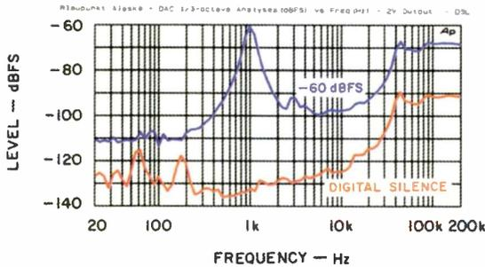
Fig. 11—Noise analysis, D/A converter.
