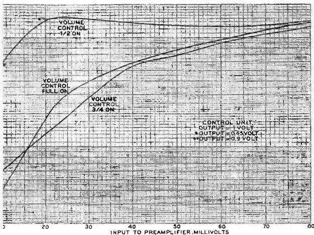
Fig. 11. Distortion on low-level inputs, as a function of input voltage, for three positions of volume control.
