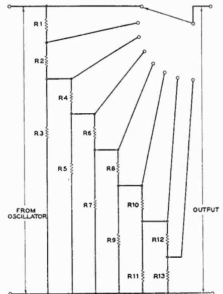
Fig. 7. The output attenuator section.
