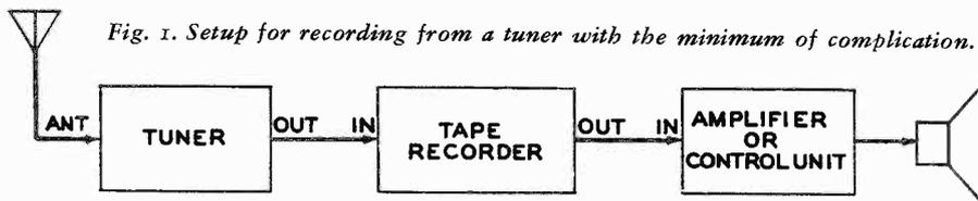
Fig. 1. Setup for recording from a tuner with the minimum of complication.
