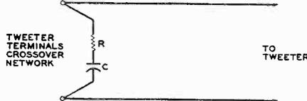
Fig. 1. Peak-suppressor for a tweeter.
