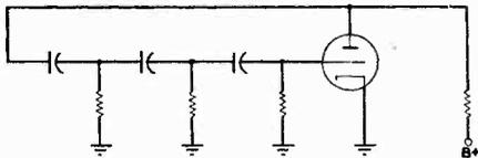
Fig. 3. Phase shift by an RC network.
