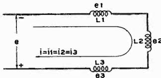
Fig. 1. Series inductors add directly.
