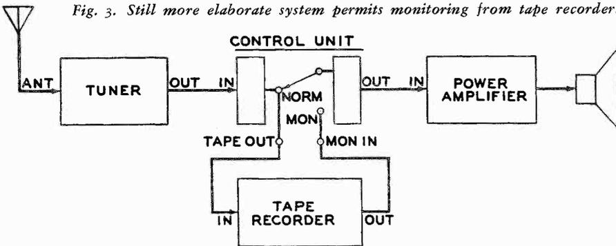
Fig. 3. Still more elaborate system permits monitoring from tape recorder.
