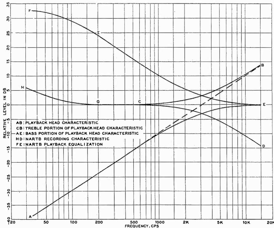
Fig. 8. How flat over-all response is achieved with optimum signal-to-noise ratio.
