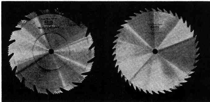
Above: hollow-ground blade for circular saw. Far right: combination blade, most popular in home shop. Below: crosscut blade. Far left: ripping blade.
