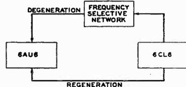
Fig. 5. Adjustable-frequency oscillator.
