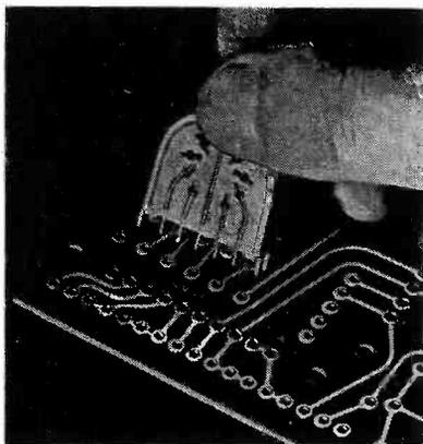
*Aerovox tube socket for printed wiring.*
