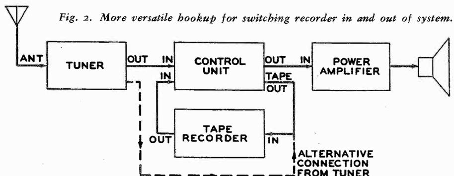
Fig. 2. More versatile hookup for switching recorder in and out of system.
