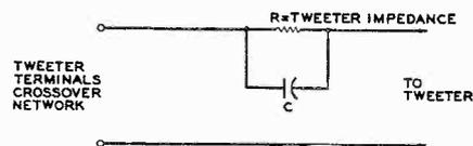
Fig. 2. High-frequency response booster.
