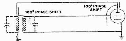
Fig. 2. Basic circuit for an oscillator.
