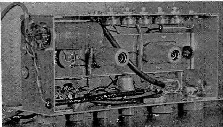
Fig. 6. Completed preamp with its outer shell removed. Note shock-mounted chassis.
