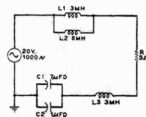
Fig. 6. Circuit for the problem example.
