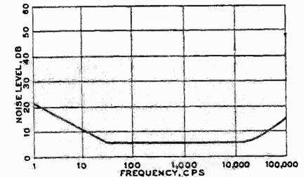
Fig. 21. Noise in very good transistor.
