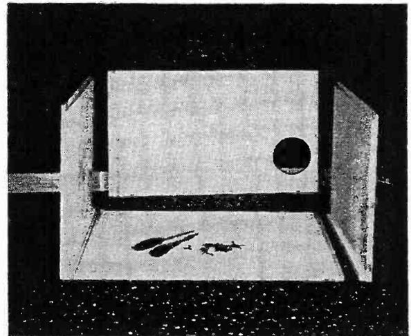
2. Put the top down on a rug, or other clean surface, and attach side pieces. Be sure all pieces face the same way; you can tell by the holes along one edge, which will be used later for front frame screws. Piece against wall is bottom.
