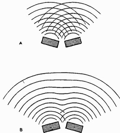
Fig. 5. For monaural sources, divergent speaker positioning was most pleasing.
