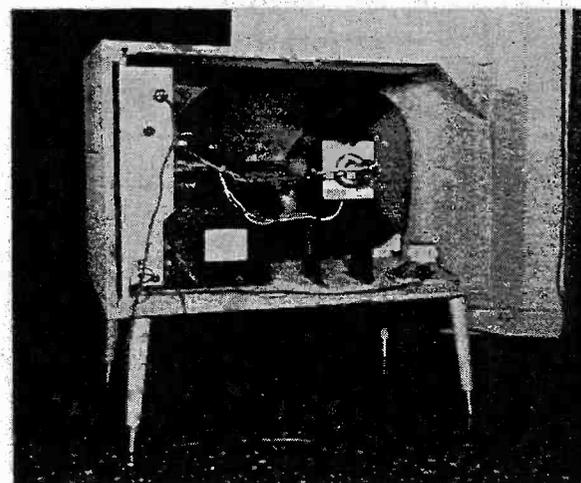
14. Everything done! Tube in, chassis in, speaker mounted. Check all wires, turn it on, tune it up; after final picture-tube and tuning adjustment have been made, the protective back piece can be added. Cabinet finish? Suit yourself!
