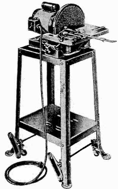
Fig. 5. The 12-inch Delta disc sander is also adjustable for many types of work.
