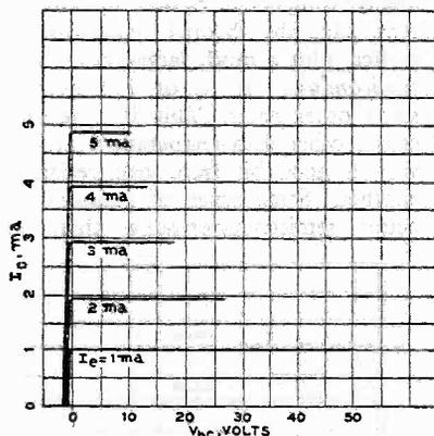
Fig. 13. Grounded-base collector curves.
