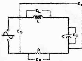
Fig. 1. A simple RLC series circuit.
