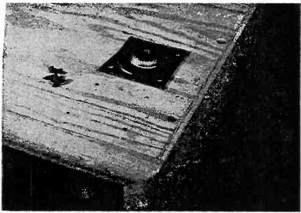
5. Attach the leg plates to the bottom. The legs must aim outward; the plates therefore tip slightly. Double check before screwing down; the cabinet is heavy and you will not want to up-end it to redo a leg plate! Note pilot holes.
