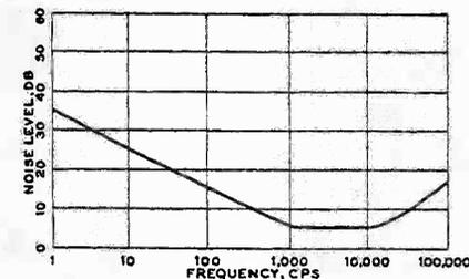
Fig. 20. Noise in fairly good transistor.
