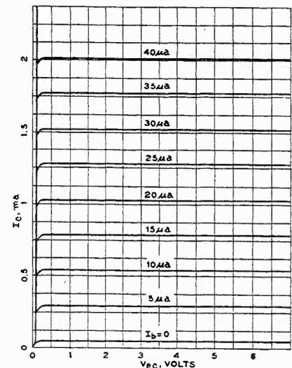
Fig. 17. The low-power collector family.
