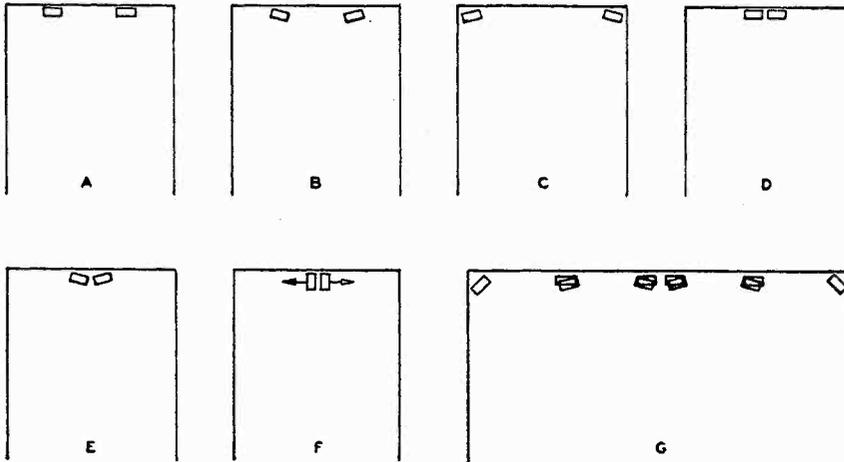
Fig. 4. Experimental positions for stereo speakers. Placement E was judged best.
