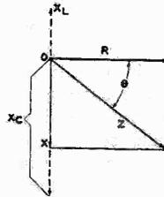
Fig. 5. Impedance vectors for Fig. 1.
