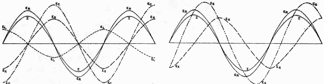
$E_c$  is larger than  $E_L$ , the total reactance is capacitive; if  $E_L$  had been larger than  $E_c$ , then the circuit as a whole would have been inductive. As would be expected, since  $E_x$  is slightly larger than the net capacitive voltage  $E_x$ , the resultant or source voltage lags the current by something less than  $45^\circ$ , and it is less than 1.414 times  $E_B$ .
