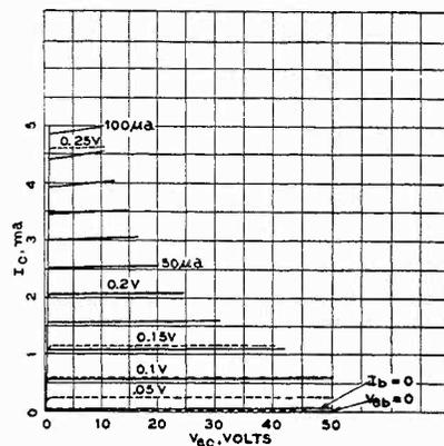
Fig. 16. Collector curve family, with both  $V_{be}$  and  $I_c$  as running parameters.
