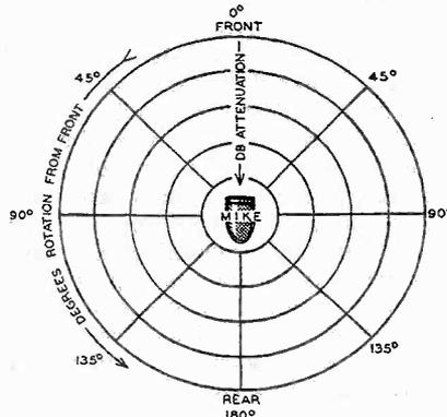
*Omnidirectional microphone is equally sensitive to sounds from any direction.*
