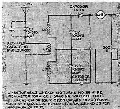
Fig. 4. Push-pull version of the tuned radio-frequency rectifier power supply.
