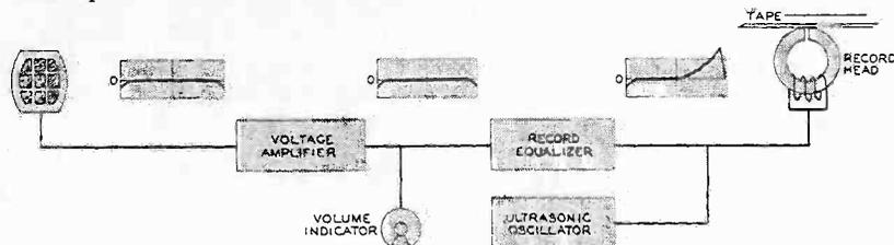
Fig. 1. Signal response at several points in recording circuit of a tape machine.
