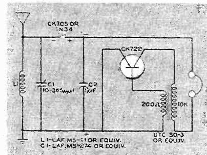
Fig. 2. A transistor audio oscillator operated by "free-energy" power supply.
