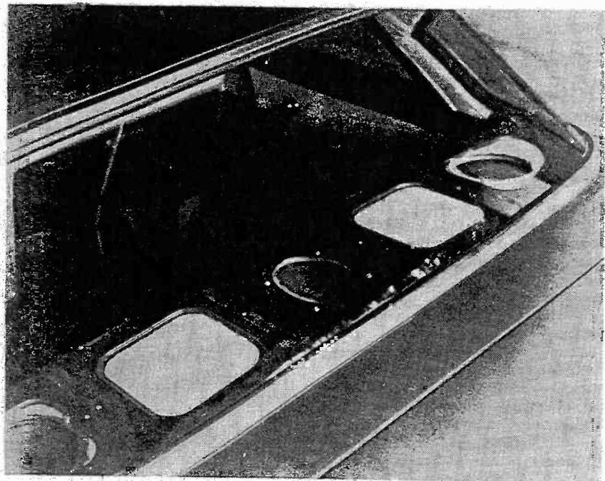
*Three speakers installed on the package shelf, ready for the first test. The glass-wool batting deadens panel resonances and makes inexpensive speakers sound almost like hi-fi units.*
