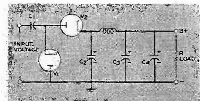
Fig. 4. A basic voltage-doubler circuit.
