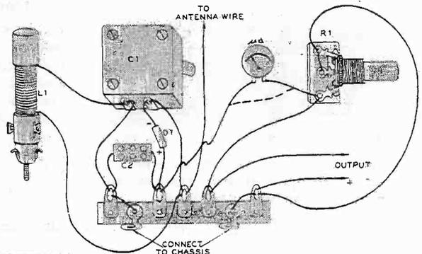
Fig. 1C, below: This revised circuit has a filter to remove AC from the DC output terminals.
