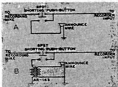
Connections for tape-recording announce mike. Circuit A is for high-impedance, and circuit B for low-impedance mike.
