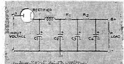
Fig. 3. Multisection power-supply filter reduces  $B+$  ripple to negligible value.
