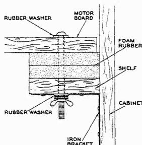
Level as it appears in cross section. the bottom rubber washer. These were tightened until the board was steady.
