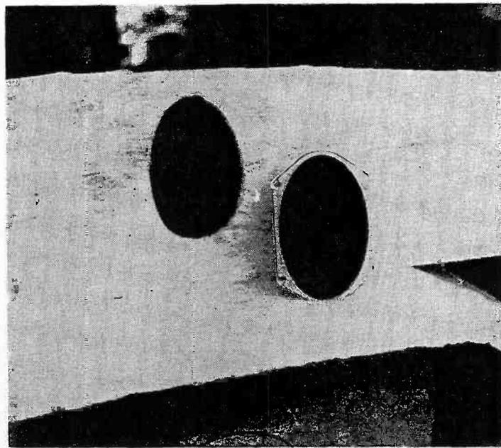
*Masonite or other hardboard is trimmed to fit below package shelf, and speaker holes cut out. Fibreglas batting of same shape is then glued to upper side of speaker mounting board.*
