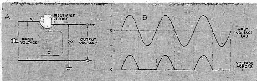
Fig. 1. A diode permits current flow in one direction only. If an AC wave form is applied, voltage across  $R$  is in a single direction: AC has been changed to DC.
