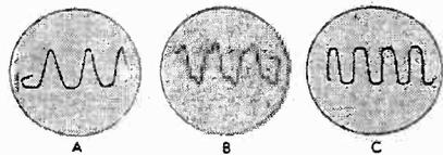
Fig. 4. Appearance of several types of distortion as seen on the oscilloscope.
