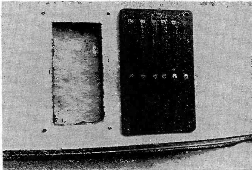
*Before installing speakers, you've marked the mounting-hole locations on lower side of the cardboard package-shelf cover. Now you can cut grille holes with a knife, and mount grilles.*
