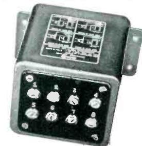
Fig. 9. This basic network provides for a wide choice of crossover frequencies.
