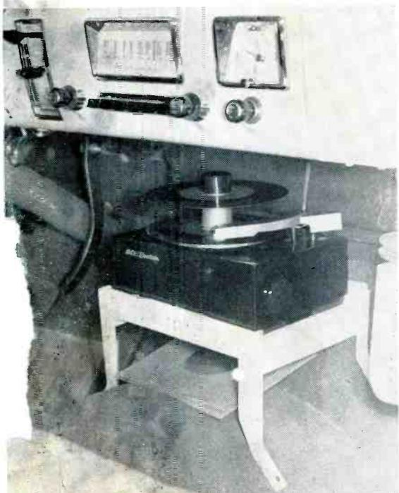
*Player fits nicely into the foam-rubber cushion, and plays through auto radio system. Power is obtained from inverter.*
