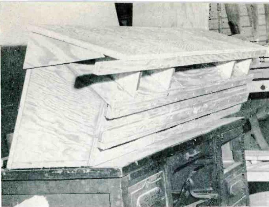
*Resonating chamber and top panel of enclosure glued and screwed together. Strip of plywood was nailed to back edges of triangular braces, and scrap pieces of plywood were attached to each end, to serve as temporary guides in positioning top panel.*
