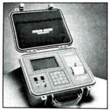
Model 1210 TDR, Cable Fault Locator
