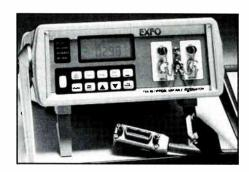
Powering is through line voltage and a built-in battery. It is said to be ideal for BER testing, ATE testing, system analysis, etc. It has linearity of  $\pm 0.05$  dB from <-3 dB to -65 dB, 0.01 dB resolution, repeatability or  $\pm 0.01$  dB. Its program mode allows up to 60 attenuation levels to be executed by the unit with a delay of one second to one hour between each allowing BER to be simplified and automated, according to the company.
