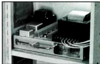
Figure 3: The SB1000 retrofits the Lectro Versatile increasing the output to 16 amps
