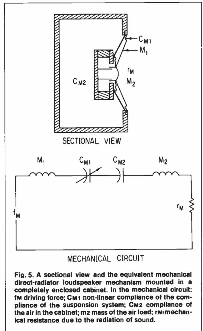
Fig. 5. A sectional view and the equivalent mechanical direct-radiator loudspeaker mechanism mounted in a completely enclosed cabinet. In the mechanical circuit:  $f_M$  driving force;  $C_{M1}$  non-linear compliance of the compliance of the suspension system;  $C_{M2}$  compliance of the air in the cabinet;  $m_2$  mass of the air load;  $r_M$  mechanical resistance due to the radiation of sound.
