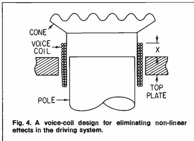
Fig. 4. A voice-coil design for eliminating non-linear effects in the driving system.
