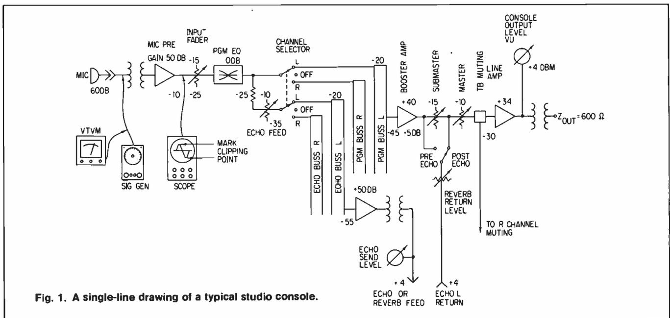
Fig. 1. A single-line drawing of a typical studio console.
