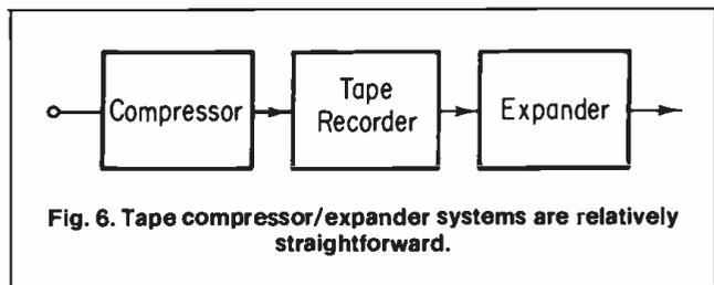
Fig. 6. Tape compressor/expander systems are relatively straightforward.
