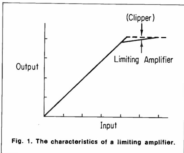
Fig. 1. The characteristics of a limiting amplifier.
