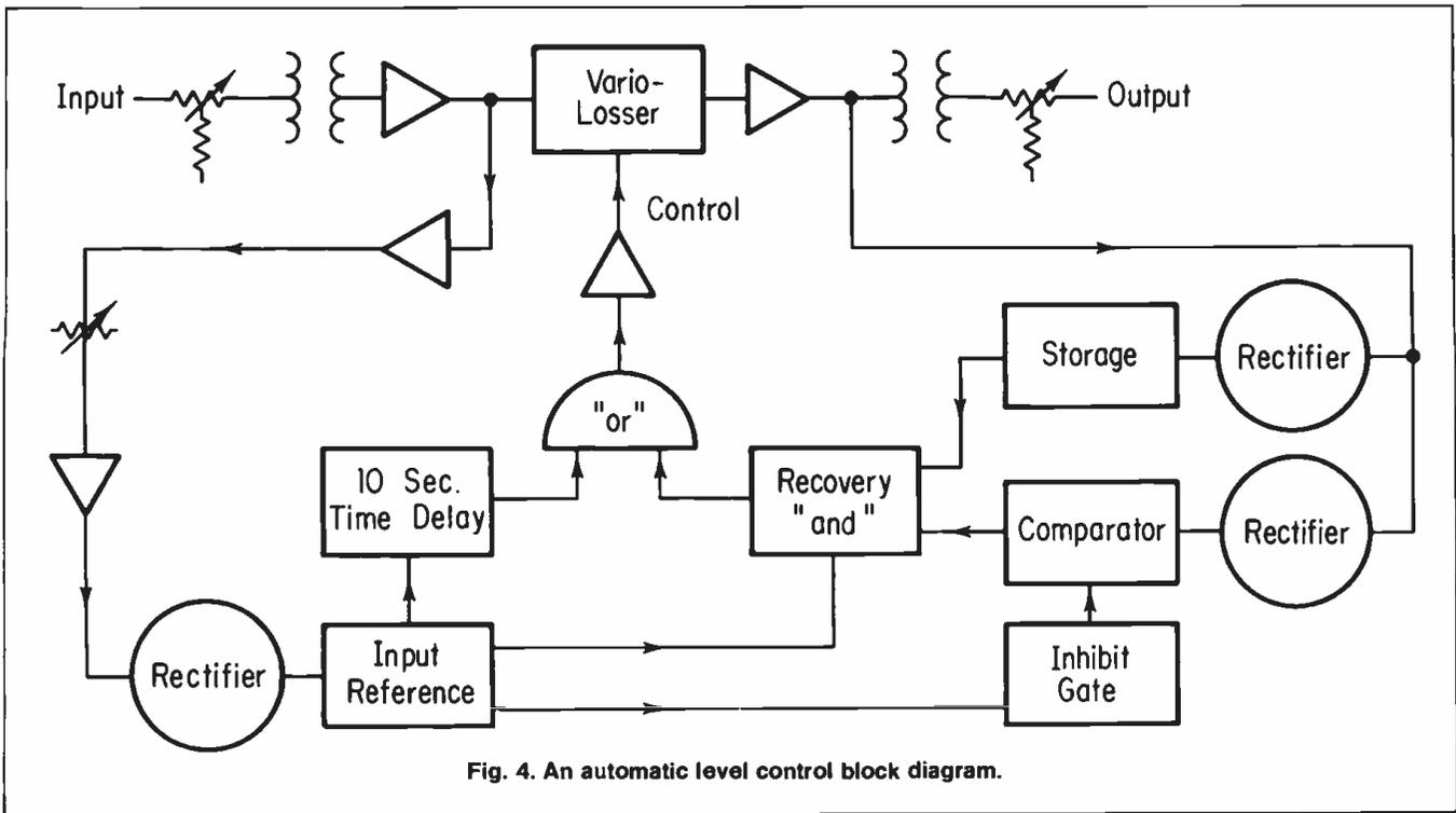
Fig. 4. An automatic level control block diagram.
