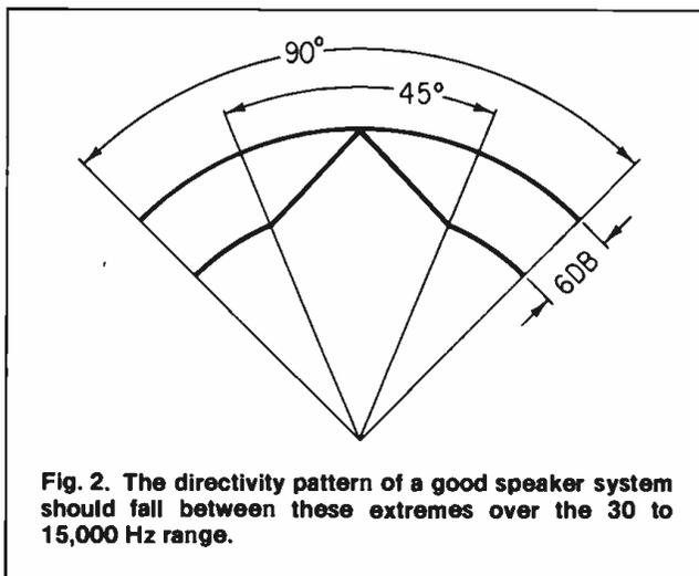
Fig. 2. The directivity pattern of a good speaker system should fall between these extremes over the 30 to 15,000 Hz range.
