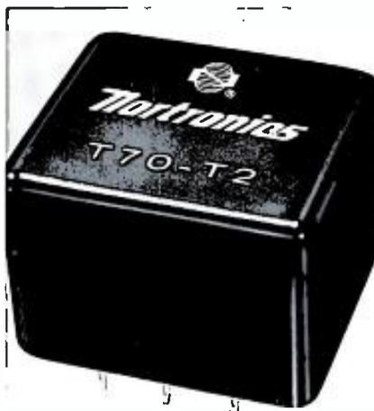
The T70-T2 bias oscillator features convenient plug-in dip-solder terminals and has the same efficient ferrite E-core construction and electrical characteristics as the popular Nortronics T60-T2 transformer. This unit will furnish up to 110 kHz of bias and erase power to full-track heads or to both channels of a stereo recorder.
