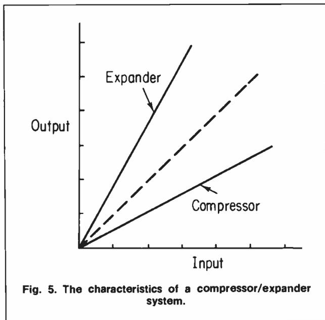
Fig. 5. The characteristics of a compressor/expander system.
