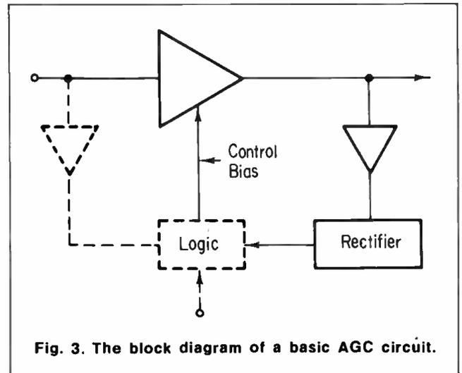
Fig. 3. The block diagram of a basic AGC circuit.
