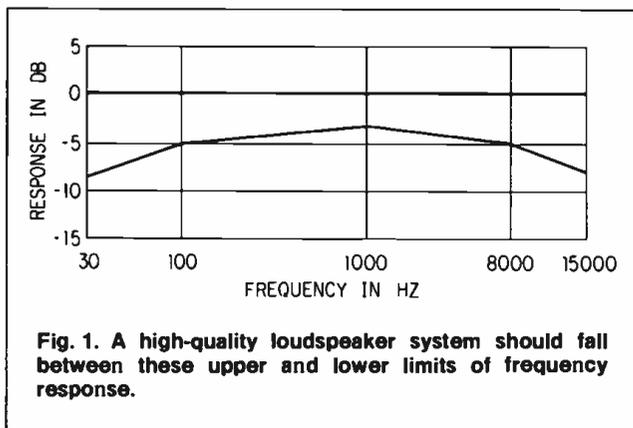
Fig. 1. A high-quality loudspeaker system should fall between these upper and lower limits of frequency response.
