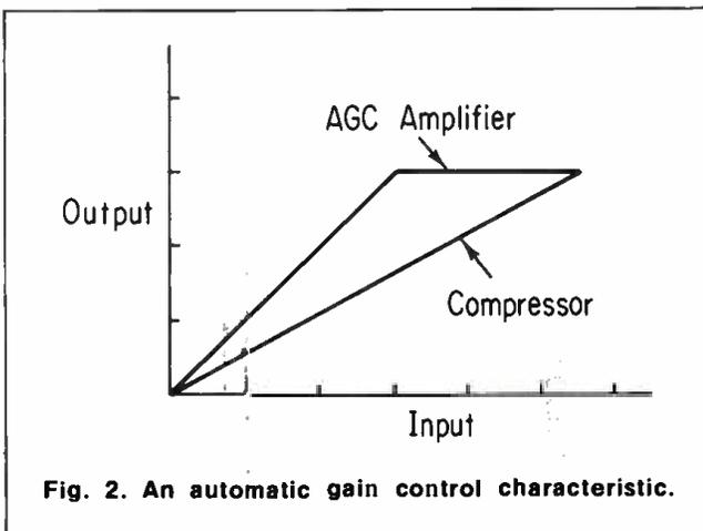
Fig. 2. An automatic gain control characteristic.
