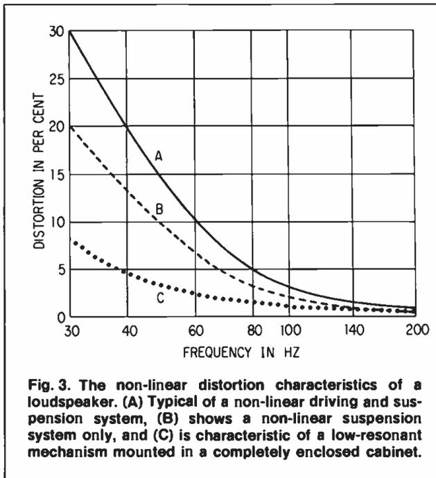
Fig. 3. The non-linear distortion characteristics of a loudspeaker. (A) Typical of a non-linear driving and suspension system, (B) shows a non-linear suspension system only, and (C) is characteristic of a low-resonant mechanism mounted in a completely enclosed cabinet.
