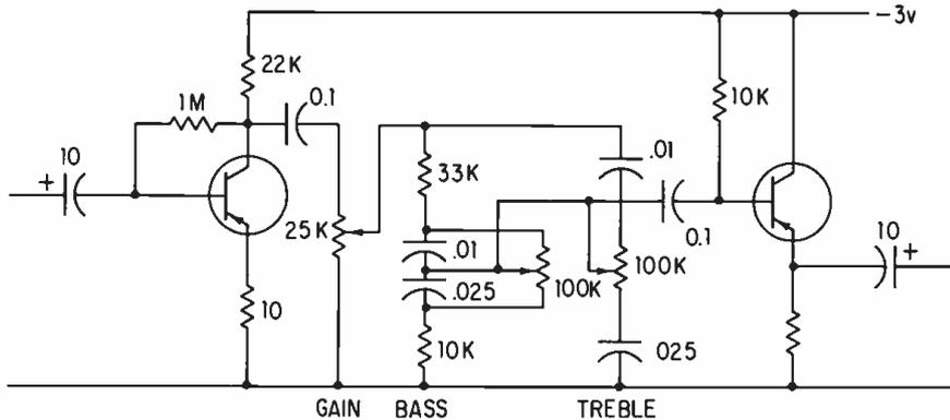
Figure 3. The final circuit that overcame the difficulties.
