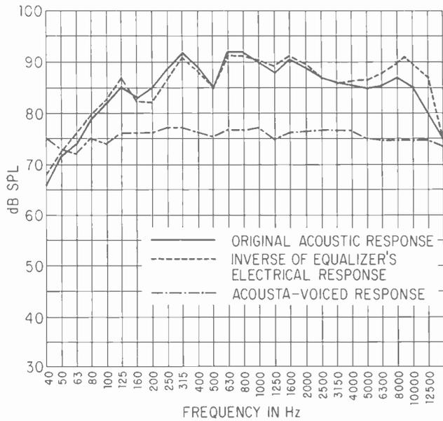
Figure 6. The result of equalizing one of the six channels. The continuous black line is the original acoustic response. The dash-dot-dash line is the Acousta-Voiced response at the engineer's ears. The dotted line reveals how closely the equalizer's inverse electrical response matches the original acoustic response.
