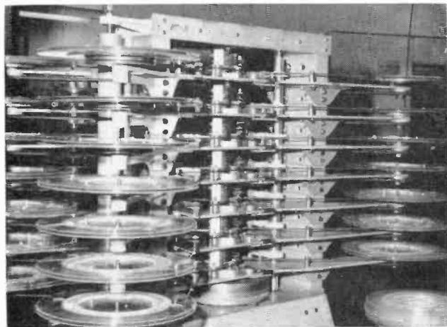
Figure 3. A single common-capstan duplicator can simultaneously run fourteen tapes. For cassettes the master speed is 120 in./sec., while the duplicator is running at 30 in./sec. All four stereo tracks are recorded in the single pass.
