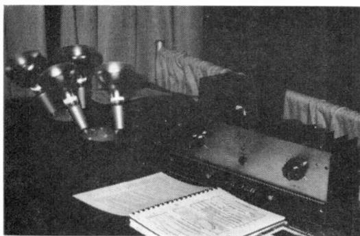
**Crown.** A dual-channel basic amplifier with a power response of d.c. to 20,000 Hz  $\pm 1$  dB at 150 watts r.m.s. per channel at an 8-ohm load. Stability is secure with all speaker loads, capacitive loads under 1 mFd, and other capacitors if isolated by 1 ohm. There is complete protection against shorts, opens, and mismatches. At 8 ohms, typical i.m. distortion is under 0.1 per cent at any level up to full power. Price: \$685. Circle 62 on Reader Service Card.
