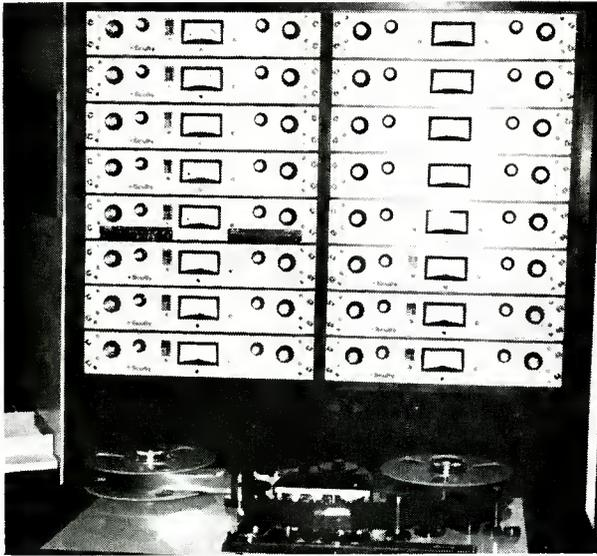
**Scully.** Sixteen tracks on two-inch audio tape with versatile control. Circle 17 on Reader Service Card.
