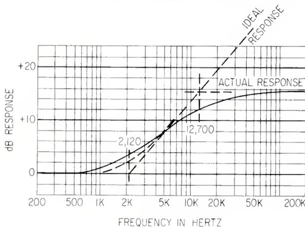
Figure 6. How the practical limitation affects pre-emphasis response. The solid-line curve is the response yielded by either circuit of Figure 5.
