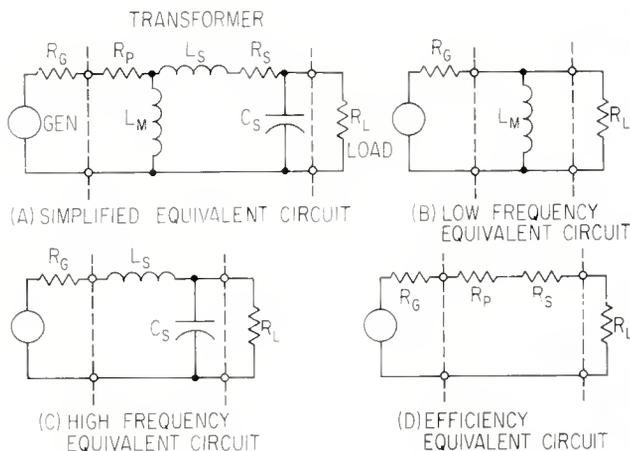
are used for isolation, impedance matching, voltage transformation, and current transformation. Voltage and current changes are a function of the turns ratio, and the power in the primary circuit equals the power in the secondary. We therefore have the well-known transformer equations:
