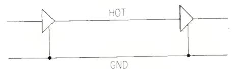
Figure 2. The unbalanced interconnection of amplifier stages.
