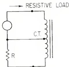
(B) GENERATOR DRIVING RESISTIVE LOAD
