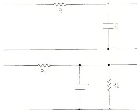
Figure 2. The essential circuit for achieving de-emphasis response. Above, in simple basic form. Below, incorporating input source resistance,  $R_1$ , and output load resistance  $R_2$ . The equivalent value of R (left) is the parallel combination of  $R_1$  and  $R_2$ .
