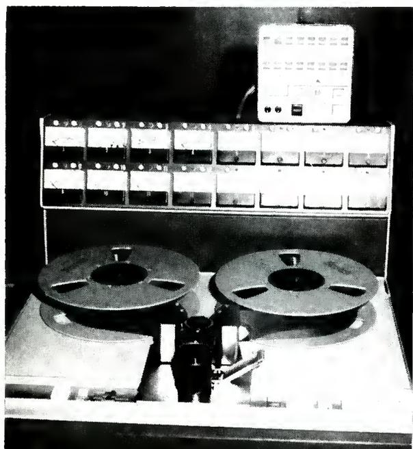
**3M Company.** Remote overdub, sixteen tracks, two-inch tape and the special tape drive system. Circle 33 on Reader Service Card.
