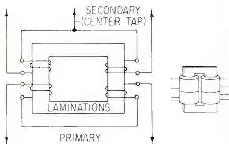
Figure 5. A balanced transformer.
