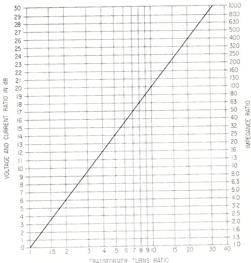
Figure 2. Transformer nomograph.
