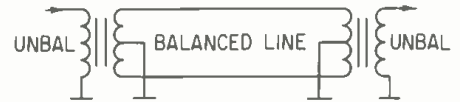
Figure 3. The use of a transformer for the conversion of a line to and from unbalanced to balanced.
