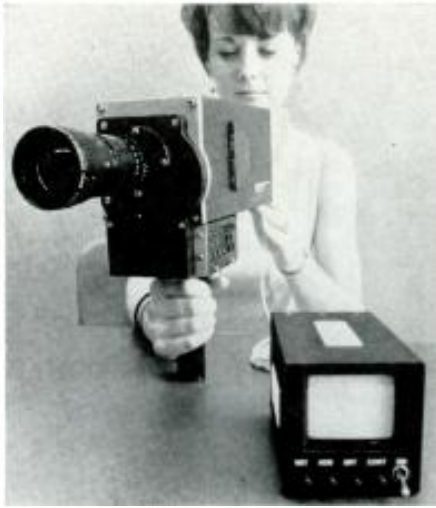
Figure 2. Apollo 10 astronauts used such a color camera to take pictures of the moon during their mission. The monitor's screen is about the size of a credit card, with the entire camera weighing less than fifteen pounds.
