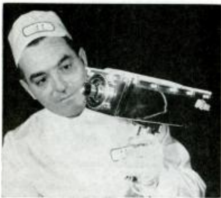
Figure 1. This is the type of television camera used by US astronauts transmitting from their craft and the moon. The camera is being held by Stanley Lebar, Westinghouse program manager, it weighs seven pounds, and uses molecular electronic functional blocks in 80 per cent of its circuitry.
