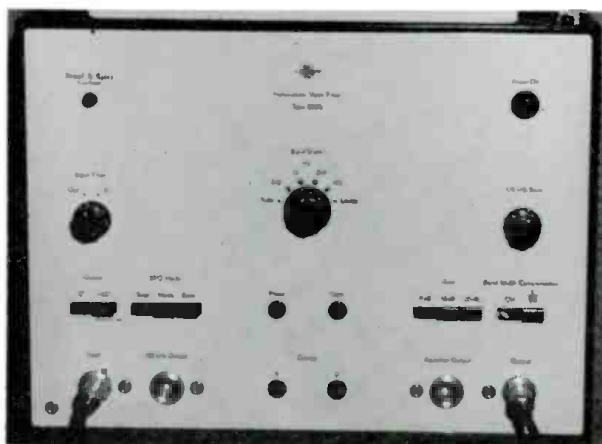
B & K. The model 2020 heterodyne slave filter may be manually or remotely controlled from 20-20,000 Hz. Circle 21 on Reader Service Card.
