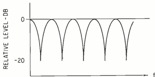
**Figure 2.** The comb-filter effect due to widely-spaced microphones. The resulting amplitude of the signal in mono shows the missing portions of the audio spectrum.
