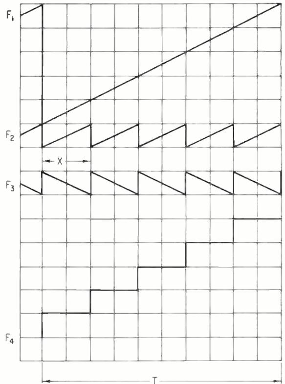
Figure 2. Constructing a step voltage using sawtooth outputs from two oscillators.
