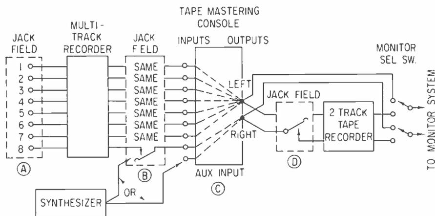
Figure 1. A representation, oversimplified to be sure, of the audio flow in a typical tape-mastering facility.
