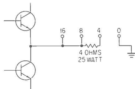
Figure 1. A method of providing multiple-impedance matching used on some earlier transistorized amplifiers.
