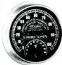
Hygrometer No. 167 is certified to be accurate within 2%. The dial indicates the complete range of 0 to 100% relative humidity and each instrument has been tested at three different positions of the dial at temperatures ranging from 32 to 230 F.
