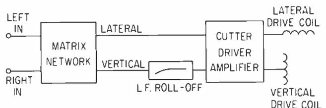
Figure 1. The Fairchild lateral/vertical stereo disc cutting system showing the signal processing in the vertical channel.
