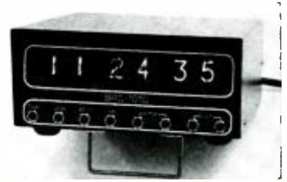
● Solid-state design is used to provide an accurate readout clock that may be used for normal clock, stop watch, or elapsed-time indication. The six-digit display gives, hours, minutes, and seconds. All operational controls are on the front panel, including start-stop and reset. The standard case is 7½ by 3½ inches, although a rack-mount is available. Options for tenth-second display, rear-projection, remote function, battery operation, etc. are available.
