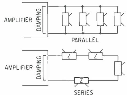
Figure 1. A comparison between parallel and series connection of speakers at an amplifier output to show the reason, based on damping, usually expressed for preferring parallel connection.
