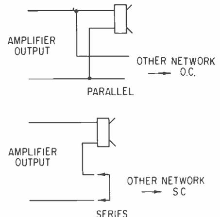
Figure 3. The actual effect of parallel and series networks does not make much difference to the coupling of damping factor to each speaker unit within its own frequency range.
