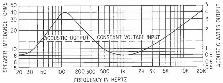
Figure 2. The effect of damping factor on frequency response. The solid curve represents a typical impedance curve. The dashed line is an ideal constant-voltage frequency response (it may not be this good). The solid curve also represents the frequency response when fed constant-current, or from an amplifier with a low damping factor.
