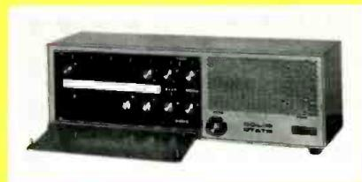
• The Pyramid Series 7000 solid-state amplifier uses two input channels to provide separate bass and treble tone adjustments for voice paging and music. As many as ten input modules can be plugged in to provide a variety of functions ranging from mic inputs to siren alarm systems. Power modules plug in also and are interchangeable in units of 20, 40, 80, and 150 watts. A limited access door is provided. Power circuits are protected by automatic devices and a visual overload alarm.
