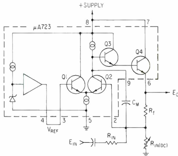
Figure 3. A  $\mu A723$  connected as an audio amplifier.
