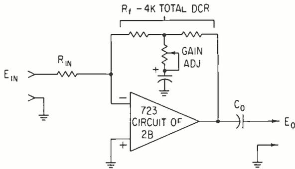
Figure 10. A configuration for adjustable gain.
