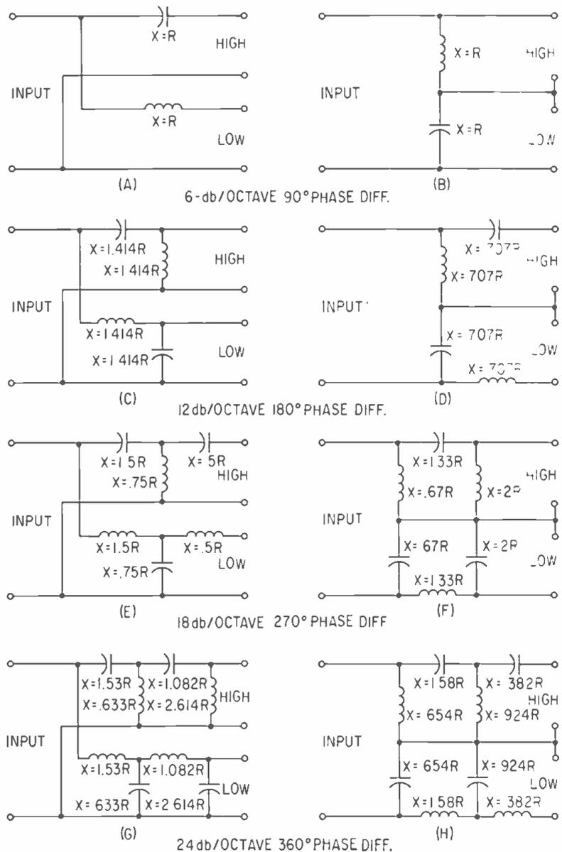
Figure 4. These are possible circuits, using from one to four reactance elements in each section to give constant resistance performance. Reactances are given in terms of terminating resistances at the crossover frequency.
