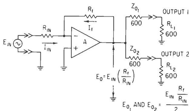
Figure 1. An opamp model of a line amplifier.
