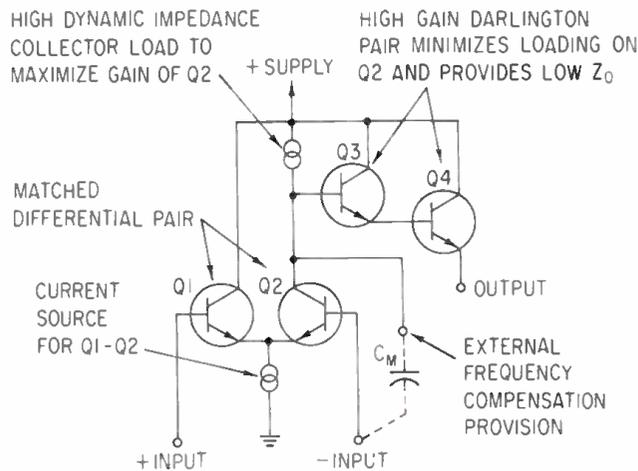
Figure 2. The circuit configuration for an IC audio amplifier.
