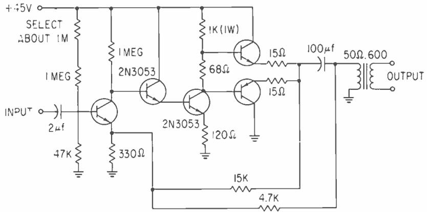
Figure 4. A line amp using discrete components.
