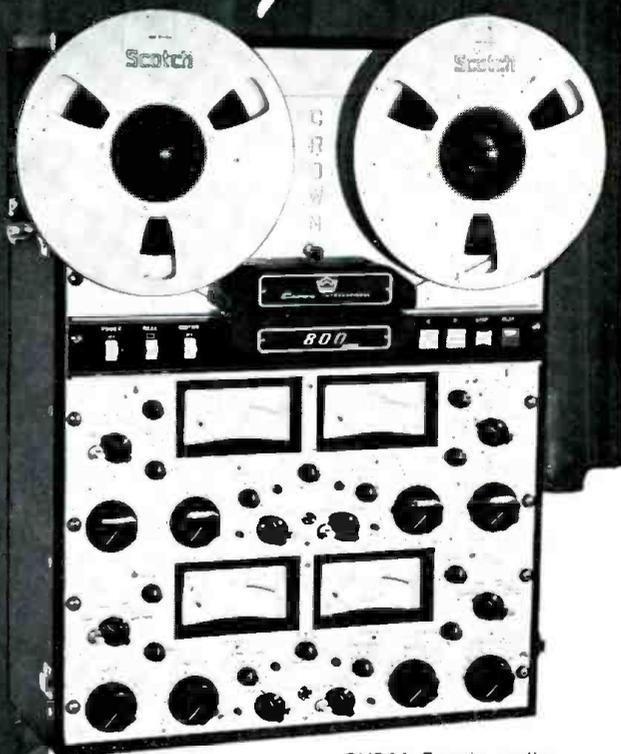
**CX844** For the audio perfectionist or professional, the ultimate in live recording. 4 channels in-line, 3 speeds, computer logic tape control never breaks tapes, remote control optional, sound-on-sound, sound-with-sound, echo effects
