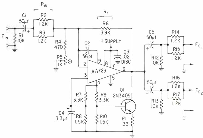
Figure 4. The complete schematic of a line amplifier using a  $\mu A723$ .
