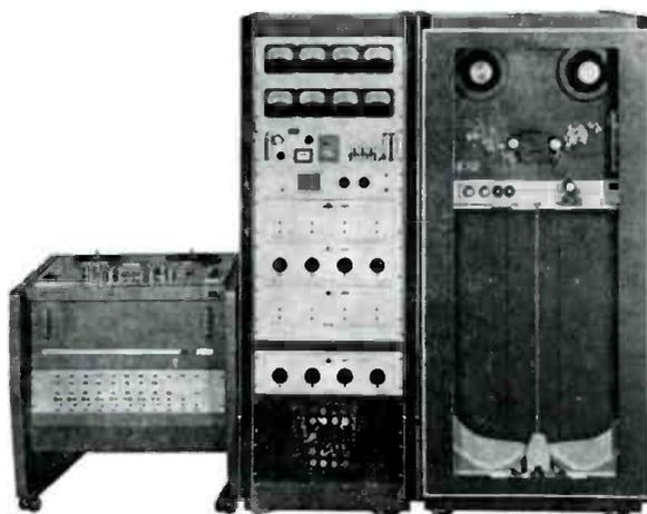
Up to 20 Slaves Complete Otari duplicating system consists of Master Reproducer with vertical endless loop bin, Logic Controller Console, and up to twenty Slave units for high volume production. Three systems available: 8-track, Cassette or Compatible System with interchangeable heads and guides.
