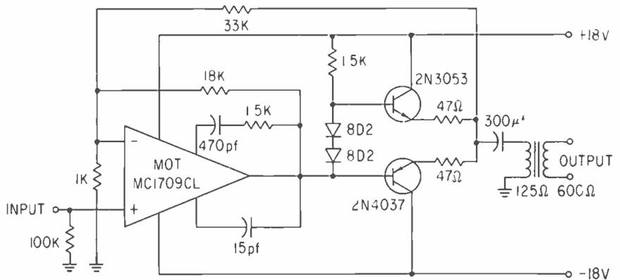
Figure 6. The line amp of Figures 4 and 5 but using the indicated integrated circuit.
