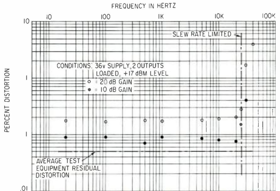
Figure 5. Total harmonic distortion at 10 dB and 20 dB gains
