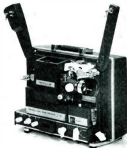
Figure 1. The Honeywell Elmo 16-S projector. It has 2000 foot capacity and still and reverse direction capability. The single button under the front of the handle sets both the automatic threading mechanism and turns on the motor.
