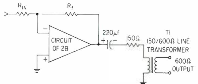
Figure 9. Alternate 600-ohm output connection for +23 dBm. You should change R11 to provide sufficient current output, and heat sinking of both the IC and Q1 is recommended. The amplifier should be labeled - - circuit of Figure 4.
