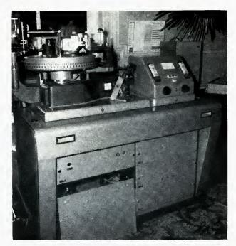
Figure 6. Crowds formed around demonstrations (as they have doen in the U.S.) of the Neumann computer-controlled disc mastering lathe, model VMS 66.
