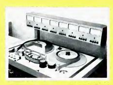
A closer view of the Pro 72, showing the tape path and head assembly section. Note that a tape timer is built in.
