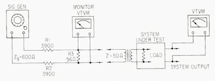
Figure 1. A balanced resistive pad for low-impedance, low-level loads.
