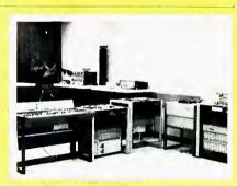
A look at part of the room. Included are a mixing desk, 1/4-inch recorders, a turntable, and a new 8-channel recorder.
