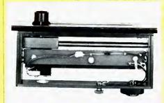
• A low-impedance straight-line ladder attenuator offers a smooth mechanical slide system. A set screw adjusts the exact tension to give a light feel. The resistive elements and related wiper mechanics are designed to eliminate contact bounce and to increase contact pressure to allow wiping through the usual atmospheric coating without making the movement stiff. The Gliss 7011 is available as a retrofit for most existing straight-line
