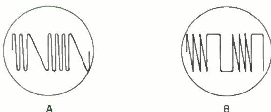
Figure 5. Examples of frequency modulation oscilloscope patterns. At (A) normal sine wave frequency modulation; at (B) a normal square wave frequency modulation.
