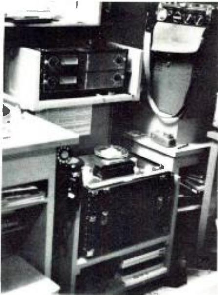
Figure 3. Have portable case, will travel. This Ampex 440 system can move to locations or serve in the studio. The Nagra at right is used for film work—a great deal of which is done at Colonial Williamsburg.
