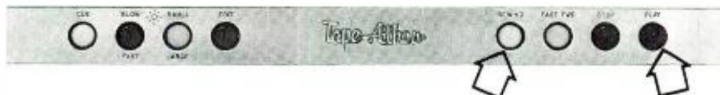
With the Tape-Athon 1001 you can initiate a "balanced torque mode" on the tape drive by activating the PLAY (or FAST FORWARD) controls simultaneously with the REWIND control. Both drive motors are balancing against one another, allowing the user to manually move the reels in either direction without drag, skipping or tape stretching. You can actually move the tape so precisely for editing purposes that splicing is virtually eliminated.
